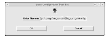
The configuration file names are unique to your target and the Ethernet device you are using. The configuration file names for your architecture are in the appropriate **target.ref.linux** file.
