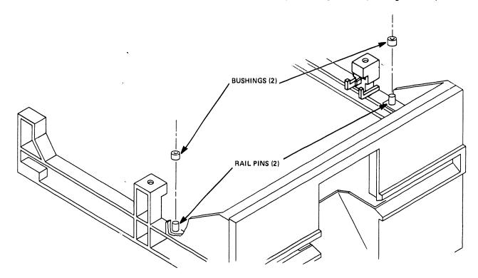
Figure 5-11 Front Panel Bushings
