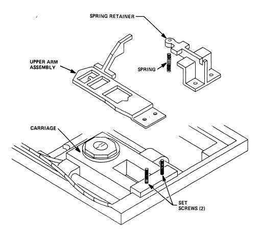
Figure 5-27 Upper Arm Assembly Parts
