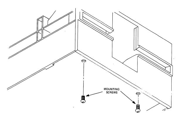
Figure 5-13 Front Panel Mounting Screws
