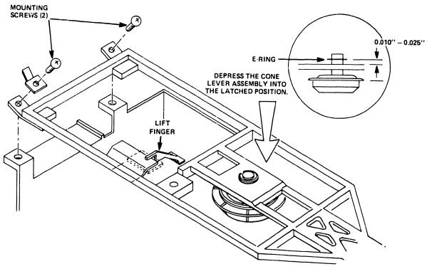
Figure 5-7 Cone Shaft and E-Ring
