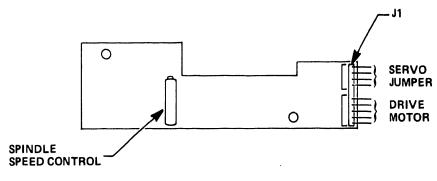
Figure 3-15 Servo PCBA
