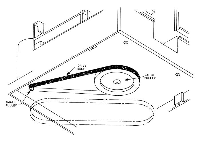
Figure 5-1 Drive Belt and Pulleys
