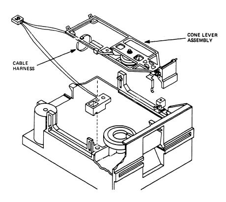
Figure 5-6 Cone Lever Assembly Cable Harness
