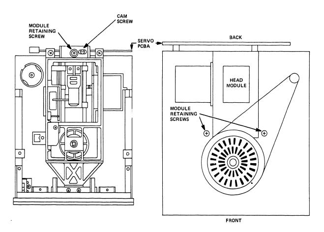
Figure 2-6 Head Module Retaining and Cam Screws
