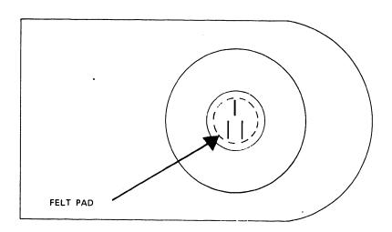
Figure 5-28 Felt Pad on Upper Arm
