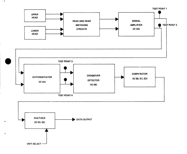
Figure 3-14 Read Circuit Block Diagram
