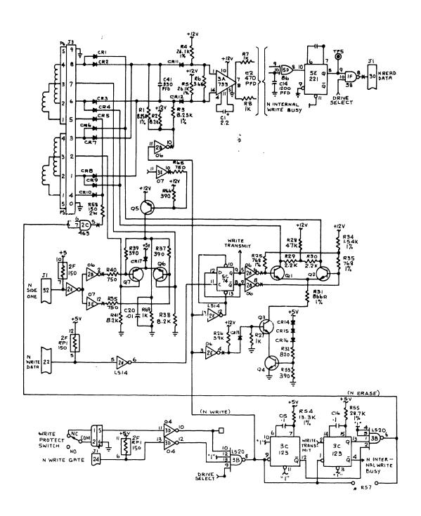
Figure 3-7 Write Data Schematic Diagram
