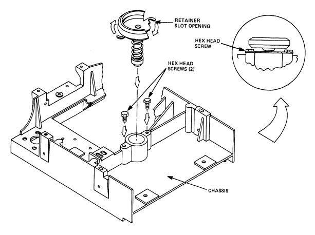
Figure 5-31 Spindle Assembly Retainer and Hex Head Screws
