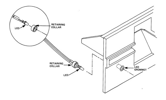
Figure 5-12 Activity LED Assembly Retaining Collar and Grommet
