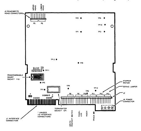
Figure 1-6 Logic Printed Circuit Board Assembly
