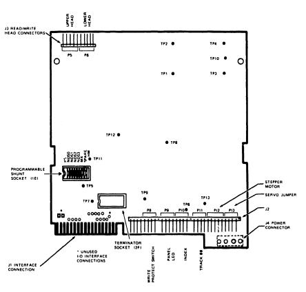
Figure 3-1 Logic PCBA
