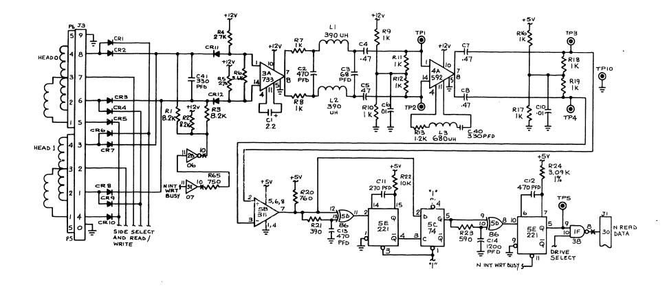
Figure 3-13 Read Data Schematic Diagram
