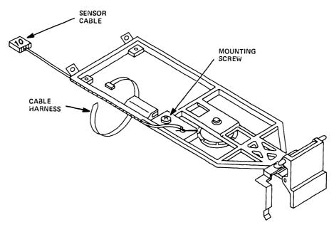
Figure 5-15 Index Emitter Sensor Harnessing and Mounting
