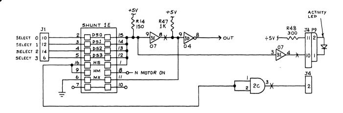
Figure 3-3 Select Lines Schematic Diagram
