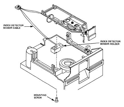
Figure 5-16 Index Detector Sensor Mounting Screw and Cable
