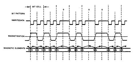
Figure 1-3 FM Recording Magnetization Profiles
