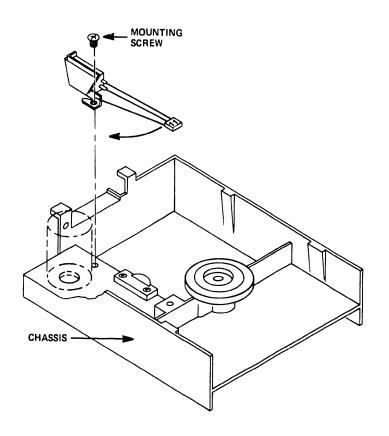
Figure 5-22 Track 00 Switch Assembly Mounting Screw
