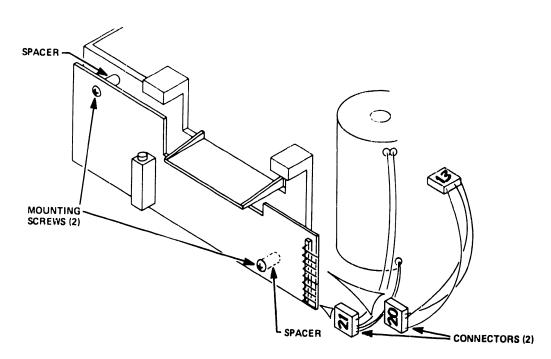
Figure 5-3 Servo PCBA Connectors, Mounting Screws, and Spacers
