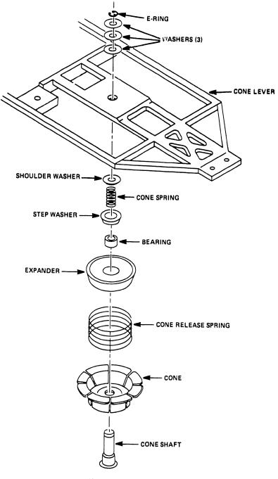
Figure 5-8 Cone's Component Parts
