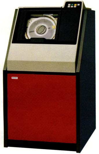
The SPERRY 5058 UNISERVO 24 Magnetic Tape Unit is offered in an additional configuration for SPERRY MAPPER 10 Systems. This tape subsystem operates using a 7-track recording format.
