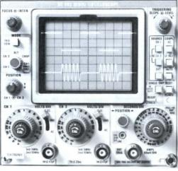
15 MHz Dual Trace Oscilloscope
