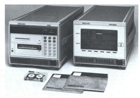
Tektronix 4041 System Controller.
