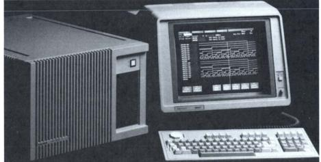
The DAS 9219 mainframe and 9200T color display form the conerstone of the 9200 Series. The mainframe supplies the 68010 CPU, 2 Mbyte system RAM, 10 Mbyte hard disk, 360 Kbyte floppy disk, three RS-232 ports, and 750 watt power supply.
