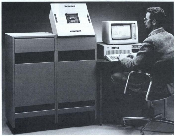
The Delta Series system occupies a minimum amount of floor space. Here, a user tests an application-specific IC (ASIC) using Tek-developed Visual Interactive Access (VIA) Software.
