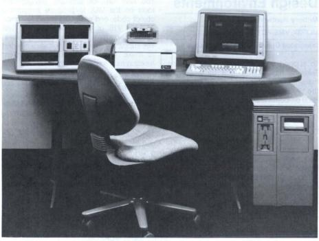
A complete software integration environment from Tektronix. Products shown from left: V1750A Software Integration Systems, 86M1750 Software Execution Unit, 4105 Color Graphics Terminal, and 8575X MicroVAX II host processor.
