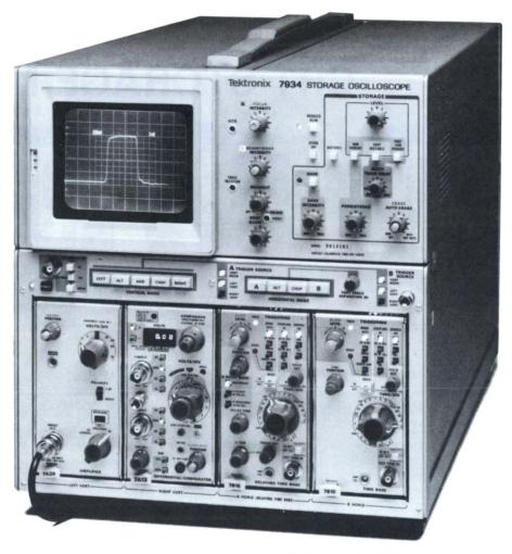
vent display erasure and provide up to 30-times extension of viewing time in the variable persistence modes . . . Auto Erase with time interval selection to more than 10 seconds between erasures.
