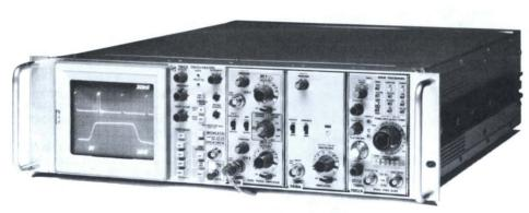
The R7903 requires only 5.25 inches of rack height in a standard 19-inch rack. It is fan-cooled and comes complete with slideout chassis tracks.
