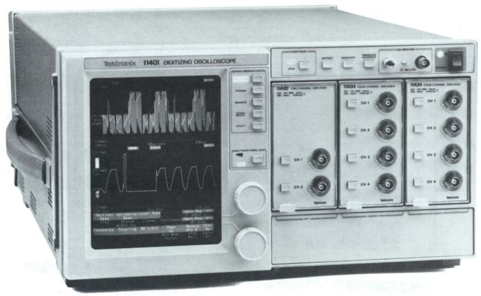
The 11401 Digitizing Oscilloscope with 500 MHz System bandwidth.
