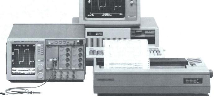
All 11000 Series oscilloscope functions are programmable via either GPIB or RS-232C interfaces. Both are standard, allowing the scopes to easily interface with PCs, workstations, mainframe computers and instrument controllers.
