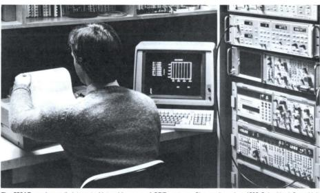
The 390AD can be easily integrated into wide range of GPIB systems. Shown above is a 4695 Color Hard Copy Unit and a 4205 Color Graphics Terminal which is connected to a Tektronix 4041 System Controller.
