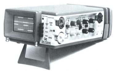
Built of impact-resistant plastic and fully self contained, this miniature portable is ideal for applications in severe environments. And it permits "floating" measurements since it is double insulated and can be elevated to 700 V (dc + ac) above ground when operated from batteries. Although insulated, normal caution should be observed when connecting the oscilloscope probe to the test point.
