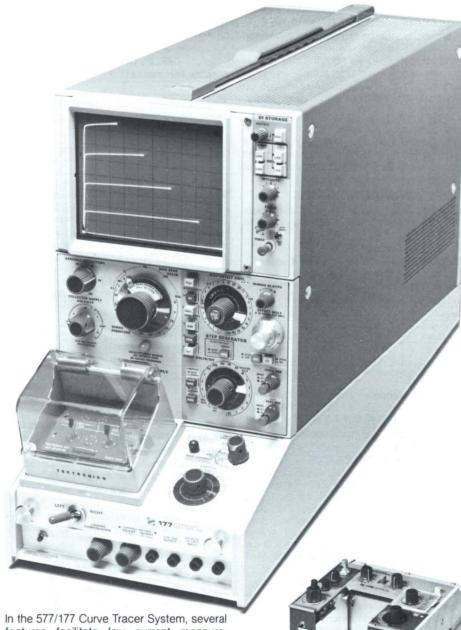
In the 577/177 Curve Tracer System, several features facilitate low current measurements. They include: small current sensing resistors (which result in less capacitive looping), current sensing that always takes place in the collector supply lead (which permits measurements on three-terminal active devices at the lowest current ranges and eliminates the need for a correction to the horizontal deflection factor), and a display filter (which reduces vertical deflection noise).
