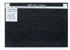
From the Main Menu, the user can select the modes of operation: SETUP, RUN, SPECIAL OPERATIONS, RE-SULTS, FILE and EDIT. Multiple drop-down menus are used to implement specific functions. Pop-up message windows provide help or indicate status.
