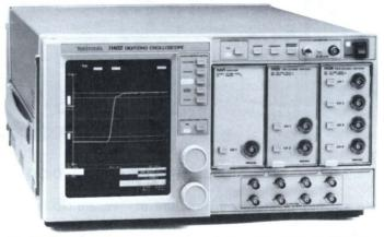
The 11402 Digitizing Oscilloscope has all of the features of the 11401 with 1 GHz maximum system bandwidth.
