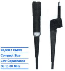
The P6055 is a miniature, low-capacitance. 10X probe designed for use with Tektronix differential amplifiers with nominal input capacitances from 20 pF to 47 pF. The attenuation ratio is adjustable to compensate for differences in input resistance of the amplifier (amplifier input resistance must be 1  $M\Omega$ ±2%). A special locking type readout connector allows use with instruments with or without readout capability.
