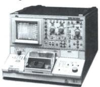
The NEW 370 Curve Tracer is remotely controllable via the GPIB for automated acquisition of curve data. Characteristic curve data can be sent in either direction over the bus. The front panel controls, except for those intended for local use only (such as Intensity), can be remotely set with a controller (like the Tek 4041) or with an IBM PC or compatible. See page 379.
