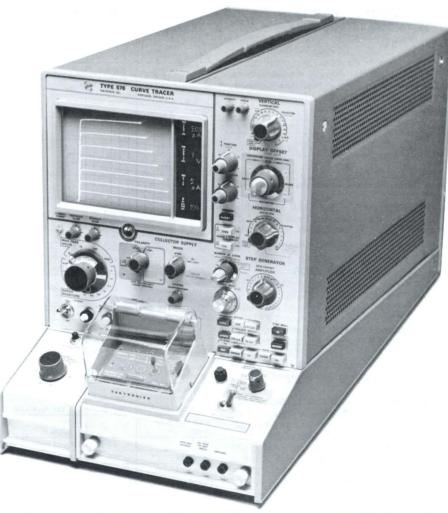
One of the features that sets the 576 apart from the Tektronix 577 Curve Tracer System is the display area adjacent to the 576's CRT. These alphanumeric indicators provide readout of vertical and horizontal deflection factors, step amplitude, and Beta/div or gm/div. The Beta or gm readout saves the operator from the arithmetic usually necessary to arrive at these parameters. These indicators also provide a permanent record of major knob settings in 576 CRT photographs.
