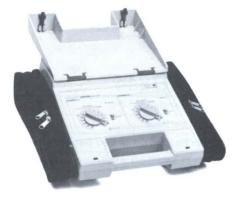
A dual-channel, optical and transformercoupled voltage isolator, the A6902B allows safely grounded test instruments to make floating measurements at high sensitivity levels in the presence of large commonmode signals.
