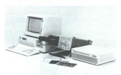
DCS01 Digitizing Camera System captures repetitive waveforms from analog scopes and transients according to a scope's CRT writing speed (350 MHz for 2467).
