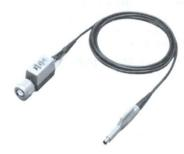
The P6125 is a low-capacitance, 5X attenuation passive probe specially designed for use with counter/timers. It makes possible more accurate time interval measurements of high speed logic signals. Five-times attenuation provides an optimum match between the counter input characteristics and the voltage levels of all common logic families. The low input capacitance permits acquisition of high frequency signals with minimum loading of the circuits under test.
