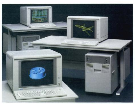
Each member of the 4120 Series is driven by an Intel 80286/80287 processor set and features a color display with Dynamic Convergence; firmware with embedded commands for segment editing, segment subroutines and pick operations; a user interactive keyboard; and 4110 and 4100A Series compatibility.
