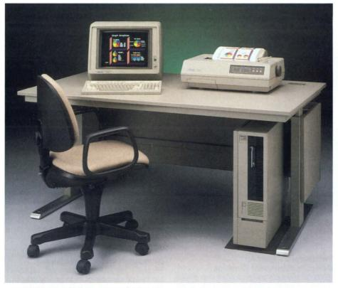
The 4132 Technical Data Analysis and Presentation System is displayed on the Tek 4107A terminal, with hard copies produced by the Tek 4696 Color Ink-Jet Printer.
