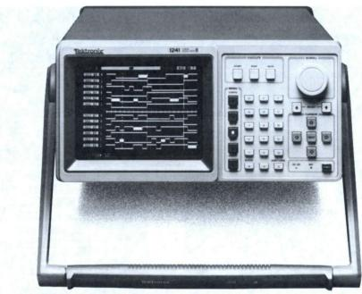
Expanded 1241 Timing Diagram With Glitches.
