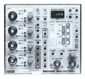
Four Channel Analog Display With Trigger View
