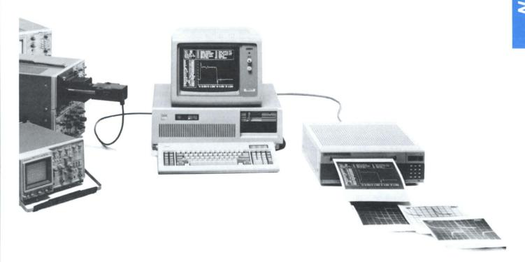
The Digitizing Camera System consists of C1001 Camera, frame store board inside the PC, DCS software, and cables. The system is shown with an IBM AT and HC02 Hard Copy Unit.
