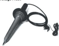
The High Voltage Probe will measure do voltages from 1 kV to 40 kV with an accuracy of 1% at 25 kV. The division ratio is 1000:1. Common uses include measuring anode voltages on monitors or oscilloscopes. Probe plugs directly into the front end of the multimeter.
