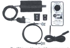
The 134 is used to extend the measurement capabilities and sensitivity of the P6021 or P6022 Current Probes. A Current/Div switch provides calibrated current steps from 1 mA/div to 1 A/div (with the oscilloscope or plug-in unit adjusted for a deflection factor of 50 mV/div). A passive termination is not required when using a 134 with a P6021 or P6022.
