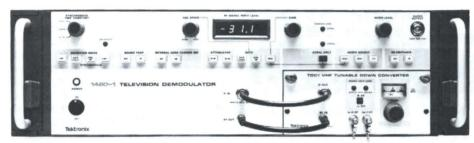
The 1450-1 is compatible with System M Television Transmission, the 1450-2 is compatible with System B/G, and the 1450-3 is compatible with System I.
