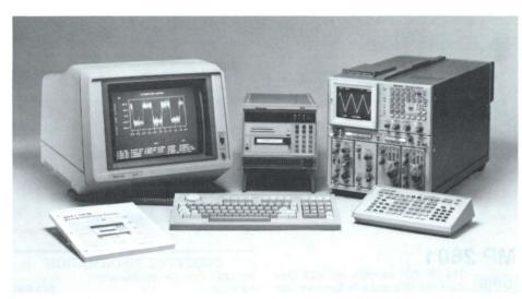
The MP 2501 Measurement Package consists of a 4205, 4041, 7854, and software.
