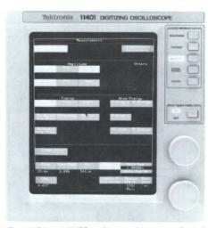
The 11401 and 11402 perform a wide range of amplitude, timing, and area/energy measurements. The measurements are automatic, accurate, easily accessible and clearly annotated for repeatable results.
