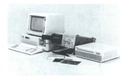
DCS01 350 MHz Digitizing Camera System pling a DCS01 Digitizing Camera System with a 2467 Oscilloscope provides a fully programmable system for digitizing repetitive or single shot events to a full 350 MHz bandwidth. The 2467/DCS combination also provides Save-On-Delta capability to detect and save that one-in-amillion deviation in a high repetition rate signal.
