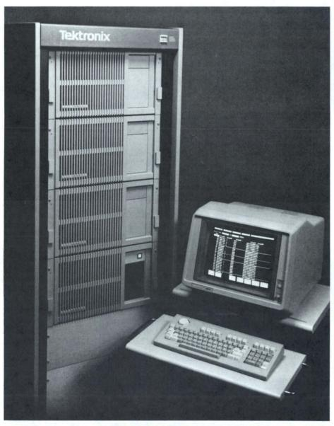
Up to three expansion mainframes can be connected to the DAS 9219 mainframe, in daisy-chain fashion, for a total of 28 slots.
