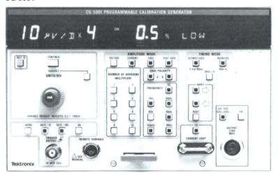
Programmable Oscilloscope Calibration Generator
