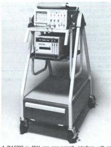
A TM 5003 or 4041 can conveniently interface with an oscilloscope on a K213 Instrument Cart. Shown with the K213 above is an MP 2601 Measurement Package. MP 2601 consists of a 4041 controller and a 2430 Digital Storage Oscilloscope.
