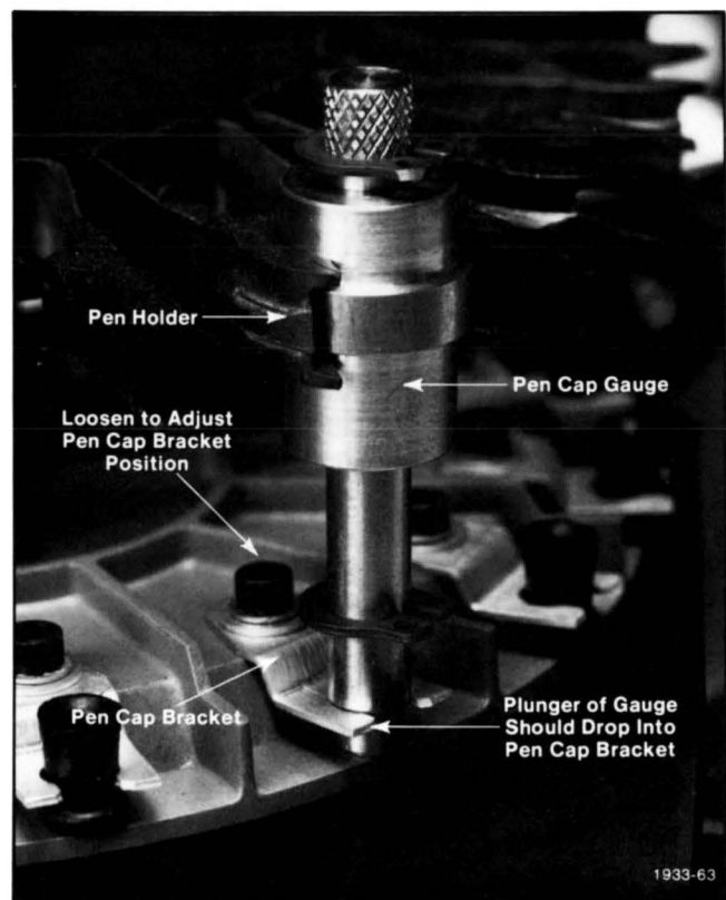
Figure 2-23. Pen Cap Alignment.
