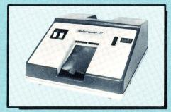
The Model 71 Duplicator is a compact, portable, table-top unit capable of producing vesicular fiche duplicates from 105mm silver masters in minimum lengths of 5 inches. A two-step duplicating process (exposure and development) is used and results in a nominal operating speed of 360, 4" X 6" fiche per hour.
