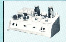
The Model 93/94 Copier is a single unit, dry-process machine capable of producing copies on vesicular film of any suitable 16mm or 35mm roll master. Film capacity is up to 1,000 feet of 3 mil copy film and 500 feet of 5.5 mil silver film. Operation speed is up to 200 feet per minute for the 94 and 120 feet per minute for the 93.
