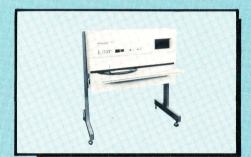
The Model 73 Duplicator is a free-standing automatic cut fiche duplicator which accepts 105mm master microfiche in any length from 5.70" to 7.40". Using either vesicular or diazo copy film high quality cut card duplicates are produced of the same size as the master. Full clearing of vesicular film is accomplished and duplicates are provided at a throughput speed of up to 800 copies per hour. Up to 99 copies of each original can be dialed into the control panel.
