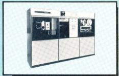
The Model 4360 converts seven- or nine-bit parallel computer data from magnetic tape into serially printed text recorded on microfilm. Alphanumeric characters are generated by the Charactron Tube. Transfer rate is 60,000 characters a second. Features include forms projection and retrieval film coding. The optional Universal Camera enables the recorder to output on 16mm, 35mm and 105mm film with a 24X, 42X or 48X reduction lens.
