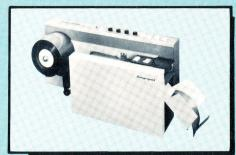
The Model 70 Fiche Cutter is an automatic 105mm roll film cutter capable of accommodating vesicular, diazo or silver films from 2 to 10 mils in thickness and in lengths from 5" to 8". Film capacity is up to 1,000 feet of roll microfiche, and operating speed is a nominal 2,500 cut fiche per hour.
