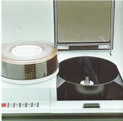
8870/2-6 workstation and data stores: cassette, magnetic disk and magnetic tape.
