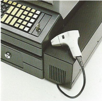
8812 computerized checkout, OCR-A-reader and integrated printer. 8862 central unit with peripherals (below).
