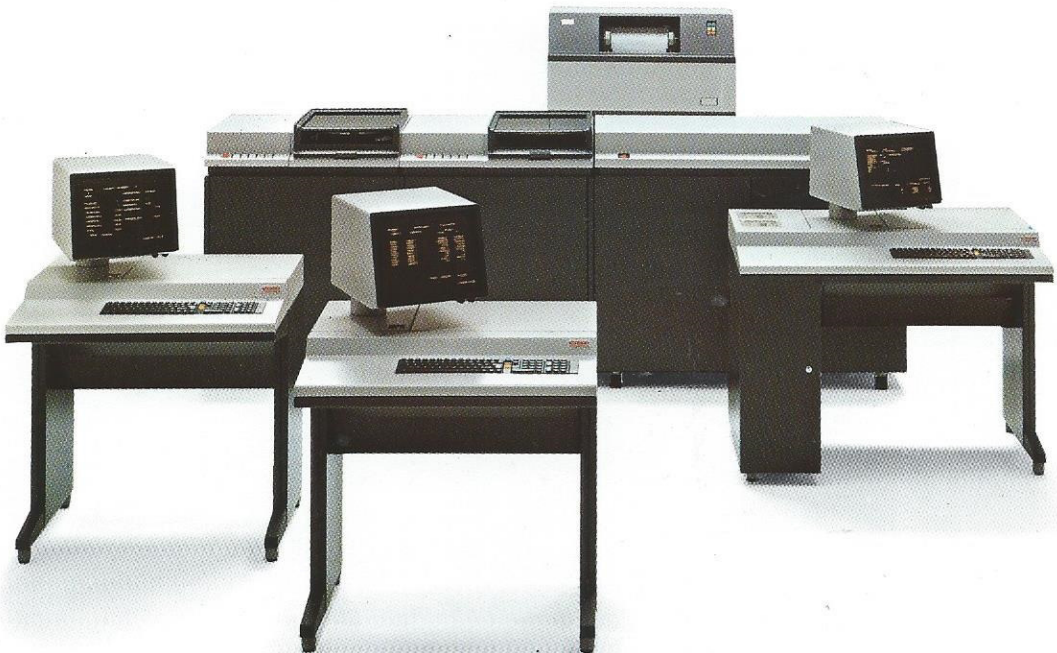
8870/2-6 workstation and data stores: cassette, magnetic disk and magnetic tape.
