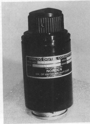
A. Photograph of shaft encoder.
