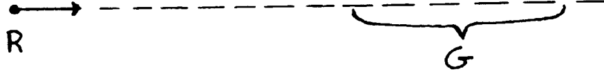
Figure 3.19. With infinite position uncertainty and perfect control, entry into the goal region is detected by observing the time sensor.
