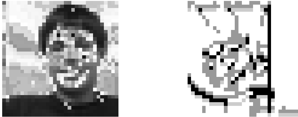
FIGURE 13-23: Test image used on 32 \times 32 processor and corresponding edges.
