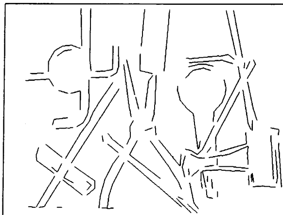
Figure 9.7: Straight line approximations to these edges.
