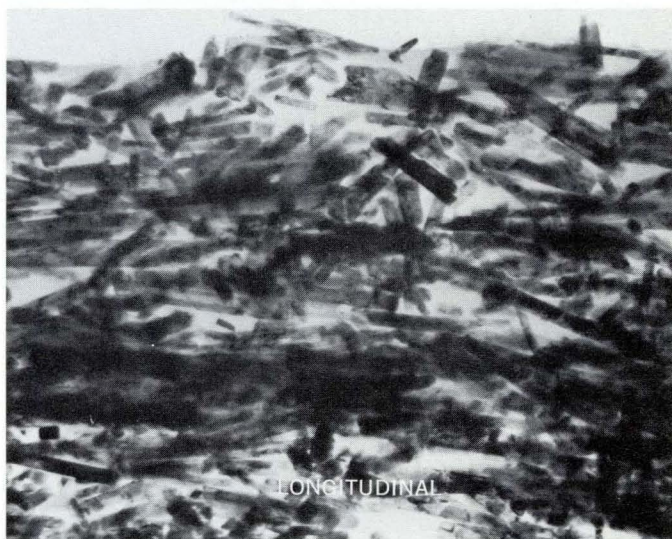
Figure 6A. Longitudinal cross-section of the magnetic oxide layer of an oriented tape (40,000X).
