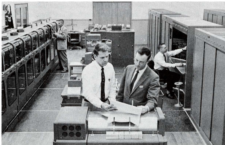
Part of the Division's $3,500,000 advanced computer center. Equipment includes the latest in high-speed digital and analog computers, including 2 Univac 1103A models.
