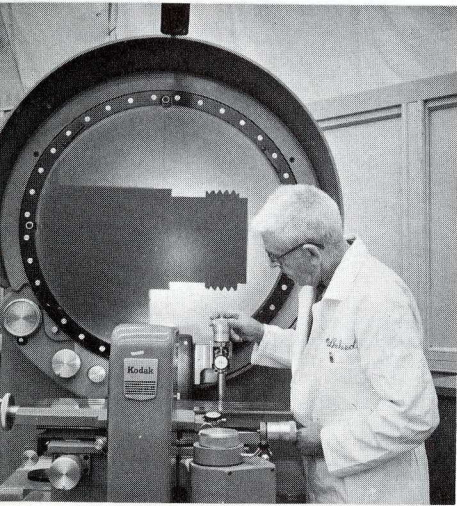
Quality assurance inspection—checking accuracy of machined threads on a 30" magnification contour projector.
