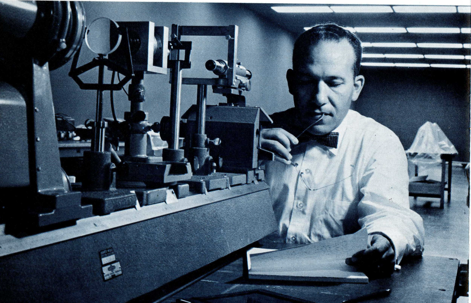
Setting up a diffraction image for a research study in near-infrared optics.
