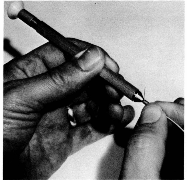
Figure 2-14. Cutting the Excess Bare Wire
