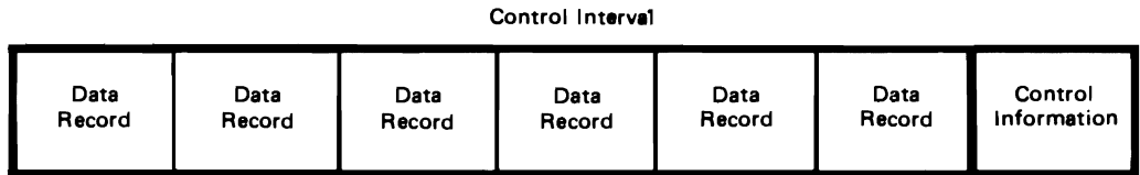
Figure 9.2 Control-interval format. Data records are stored in the front of a control interval, and control information in the back.
