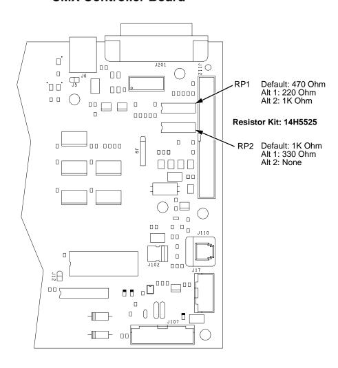
Figure 38. Terminating Resistors, Removal/Installation
