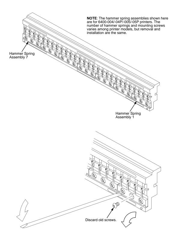
Figure 33. Hammer Spring Assembly, Removal
