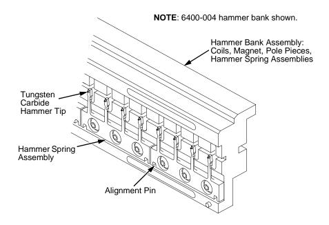
Figure 12. Hammer Springs and Hammer Bank (Detail)
