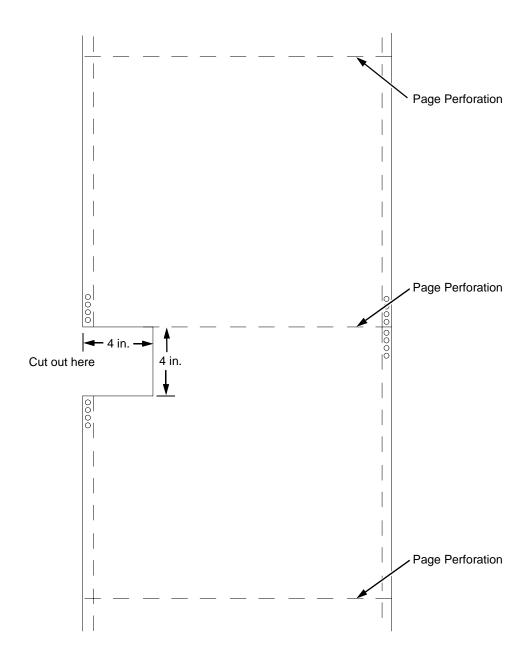
Figure 29. Paper Preparation for Paper Out Adjustment Test
