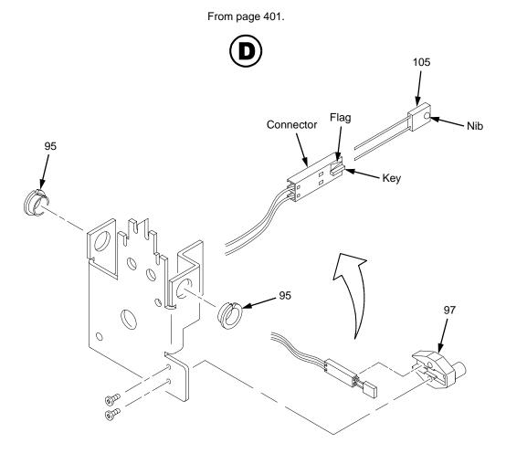
Figure 93. Stacker Detail: Elevator Bracket
