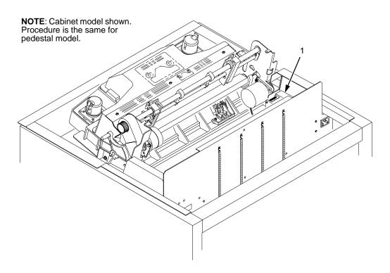
Figure 7. Cleaning the Card Cage Fan Assembly
