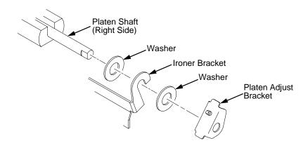
Figure 36. Installing the Platen Adjust Bracket
