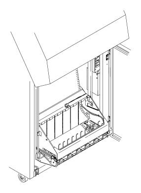
Figure 64. Power Stacker in Print Position
