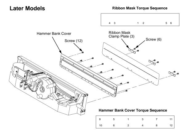
Figure 32. Hammer Bank Cover Assembly / Ribbon Mask
