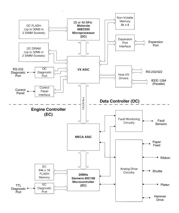
Figure 17. CMX Controller Board Block Diagram
