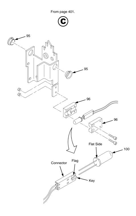
Figure 92. Stacker Detail: Motor Bracket
