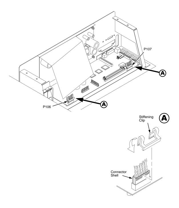
Figure 31. Connector Stiffening Clips
