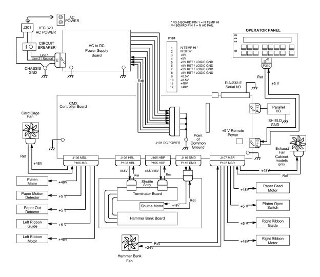
Figure 57. Ground Path Diagram
