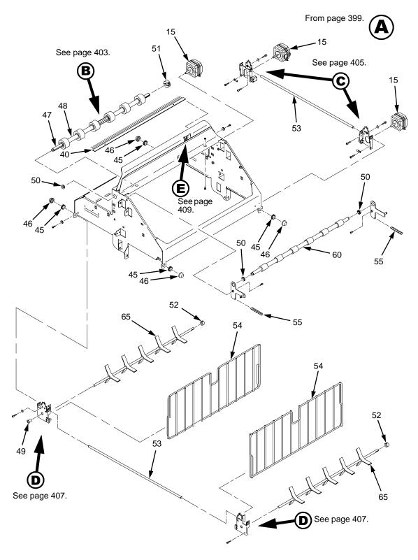
Figure 90. Stacker Detail: Motors, Rollers, and Paddles
