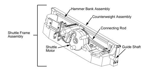
Figure 11. Shuttle Frame Assembly
