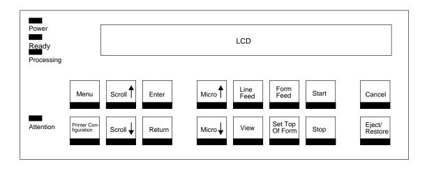
Figure 3. Electrical Controls, Pedestal Models
