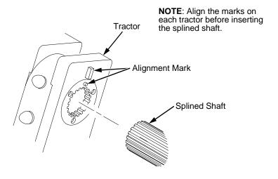
Figure 39. Splined Shaft and Tractor Installation
