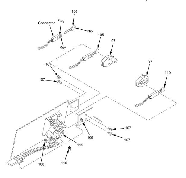
Figure 94. Stacker Detail: Paper Motion Detector
