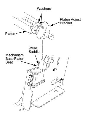
Figure 37. Positioning the Platen Adjust Brackets
