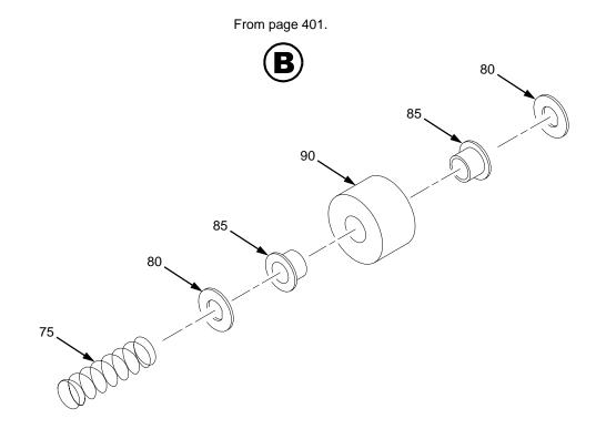
Figure 91. Stacker Detail: Rollers
