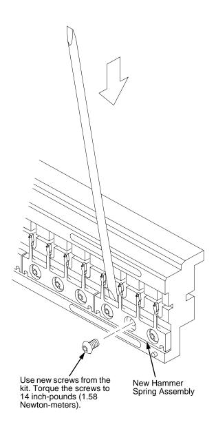
Figure 34. Hammer Spring Assembly, Installation
