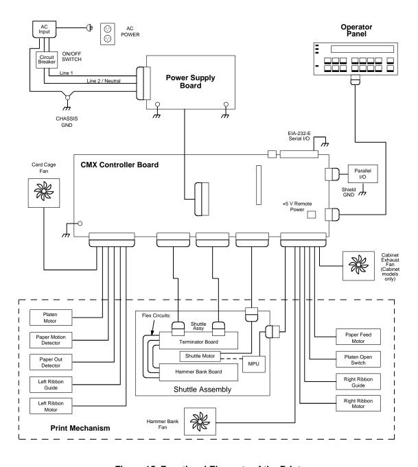
Figure 15. Functional Elements of the Printer
