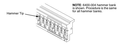
Figure 6. Cleaning the Hammer Tips
