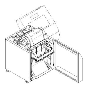
Figure 63. Paper Path in the Power Stacker
