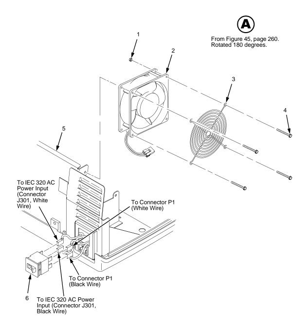
Figure 46. Card Cage Detail, Pedestal Model
