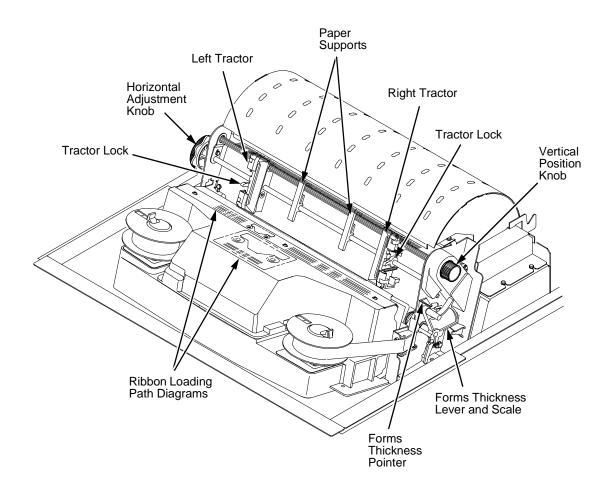
Figure 4. Mechanical Controls, All Models
