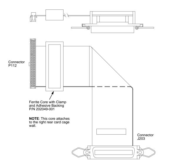
Figure 58. Ferrite Core Installation
