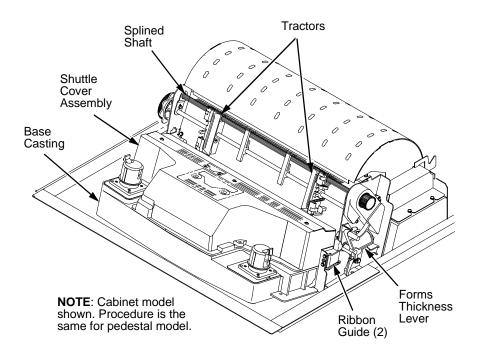
Figure 5. Cleaning Inside the Cabinet or Top Cover
