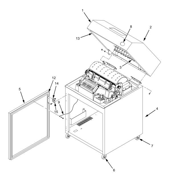
Figure 40. Top Cover, Doors, and Casters, Cabinet Model
