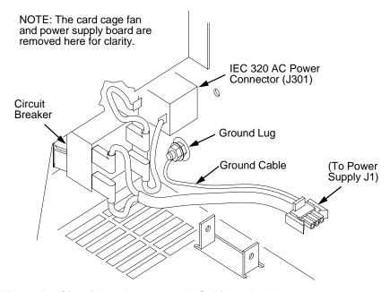
Figure 56. Circuit Breaker Ground, Cabinet Models
