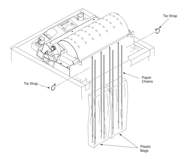
**Figure 2–9. Releasing the Paper Chains**
