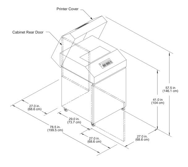
Figure 2–1. Cabinet Model Printer Dimensions
