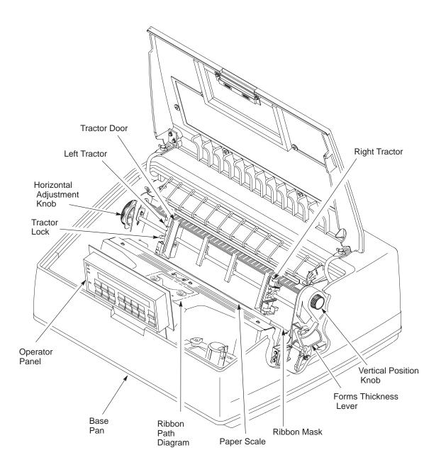
**Figure 2–4. Pedestal Model Component Locations**
