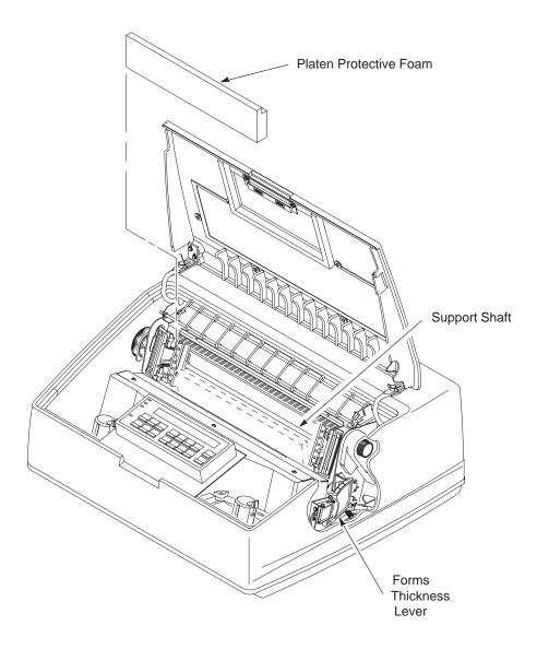
**Figure 2–12. Removing the Platen Protective Foam**
