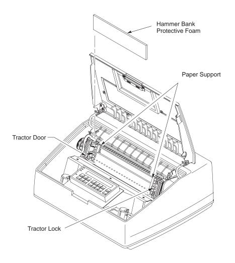
Figure 2–11. Removing the Hammer Bank Protective Foam
