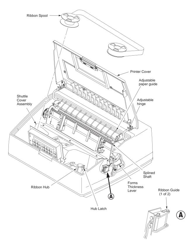
Figure 2–4. Pedestal Model Component Locations (Cont.)
