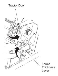
Figure 2–24. Forms Thickness Lever
