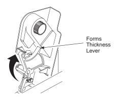
Figure 2–34. Raising the Forms Thickness Lever
