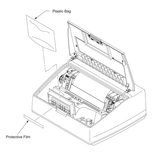
Figure 2–10. Removing the Protective Film
