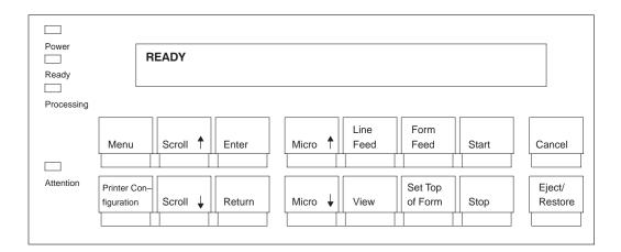
Figure 3–2. The Operator Panel
