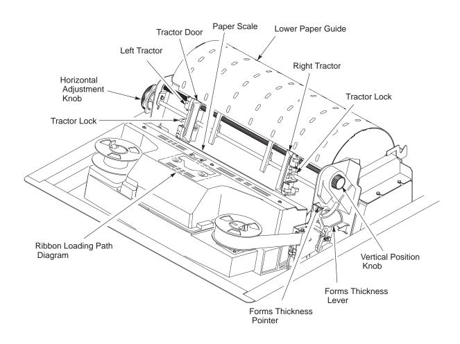
Figure 2–3. Cabinet Model Component Locations
