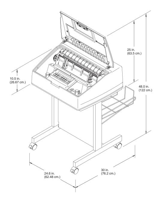
Figure 2–2. Pedestal Model Printer Dimensions
