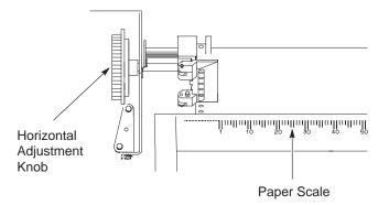
Figure 2–29. Aligning the Paper
