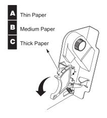
Figure 2–36. The Forms Thickness Scale
