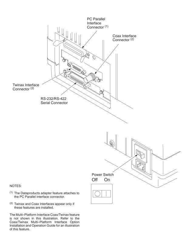
Figure 2–15. Interface and Power Cable Connections, Pedestal Models
