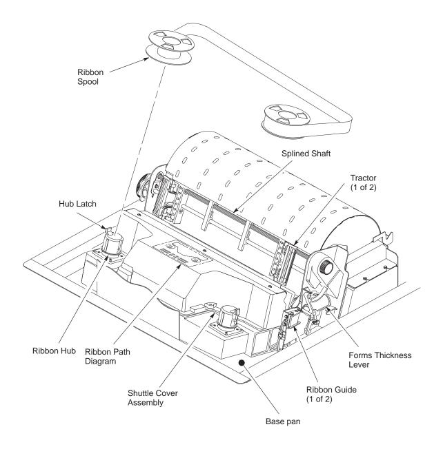
Figure 6–1. Cleaning the Printer, Cabinet Models
