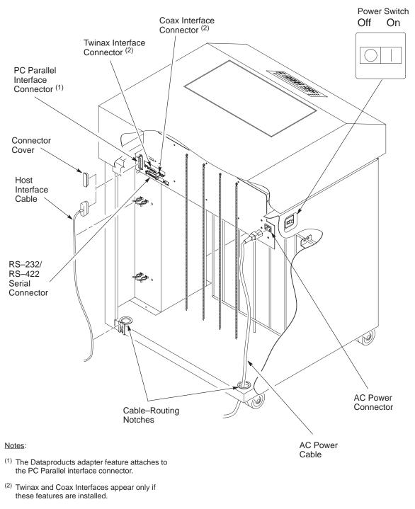
The Multi–Platform Interface Coax/Twinax feature is not shown in this illustration. Refer to the Coax/Twinax Multi–Platform Interface Option Installation and Operation Guide for an illustration of this feature.
