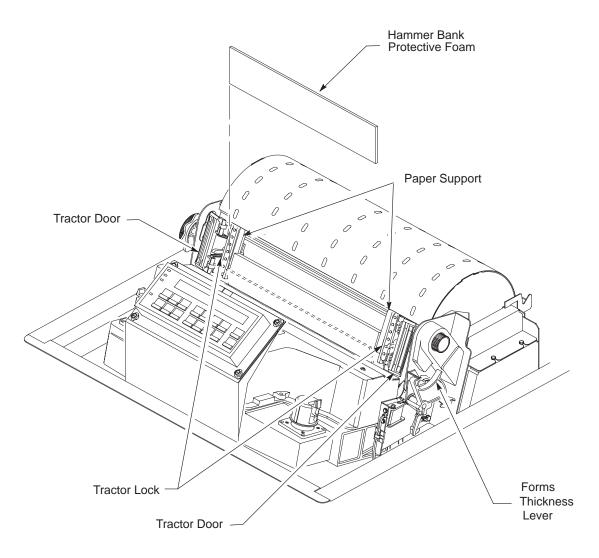
Figure 2–6. Removing the Hammer Bank Protective Foam
