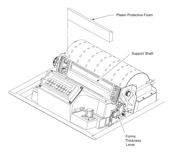
Figure 2–7. Removing the Platen Protective Foam
