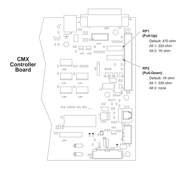
**Figure 5–1. Terminating Resistor Locations**
