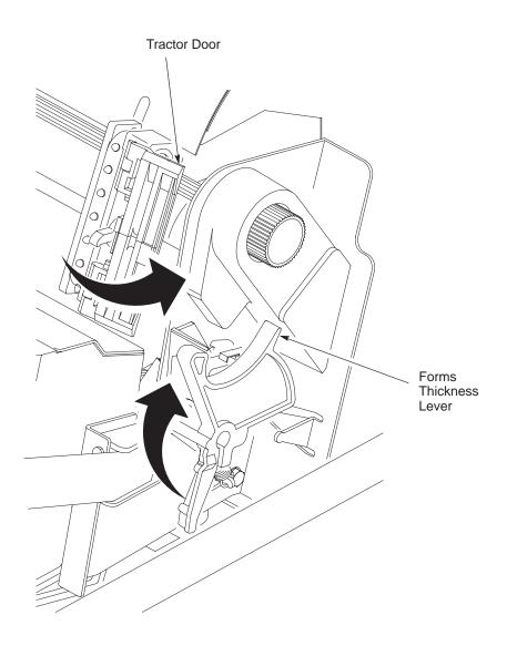
Figure 2–19. Forms Thickness Lever
