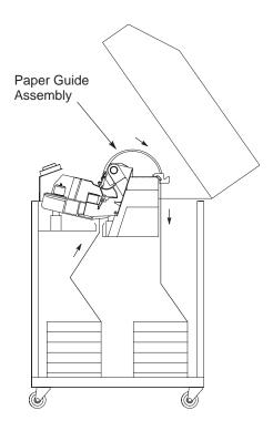
Figure 2–32. Checking the Paper Feed (Cabinet Models)
