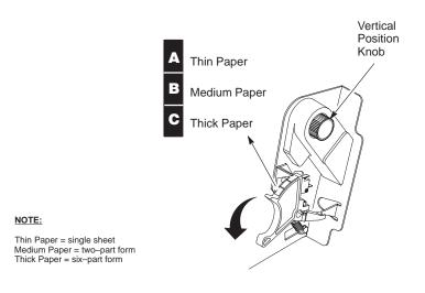
Figure 2–30. The Forms Thickness Scale
