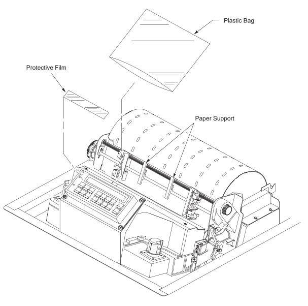
Figure 2–8. Removing the Protective Film
