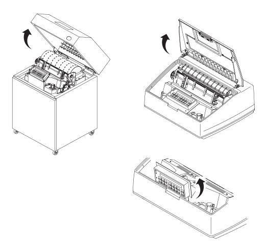
Figure 2–18. Opening the Printer Cover
