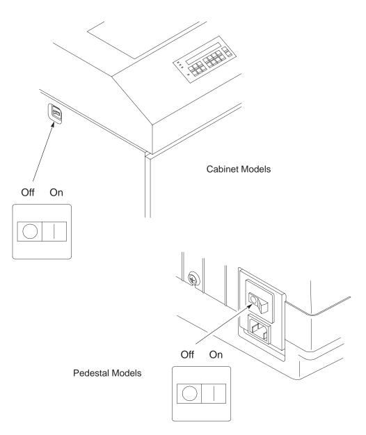
Figure 2–31. The Power Switch
