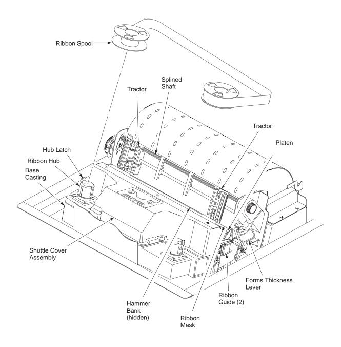
Figure 2–3. Cabinet Model Component Locations (Cont.)
