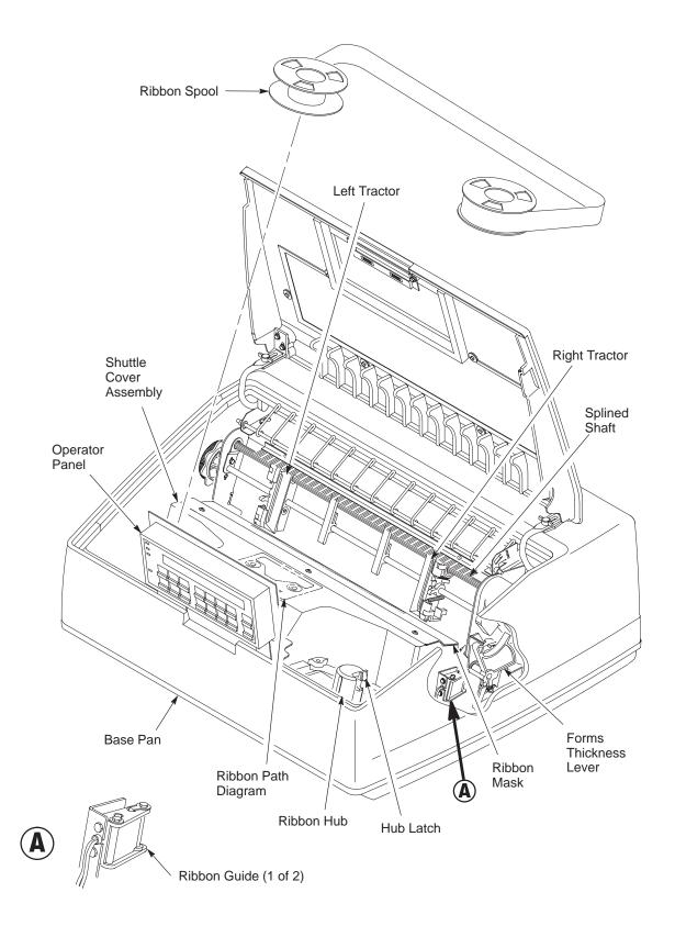
Figure 6–2. Cleaning the Printer, Pedestal Models
