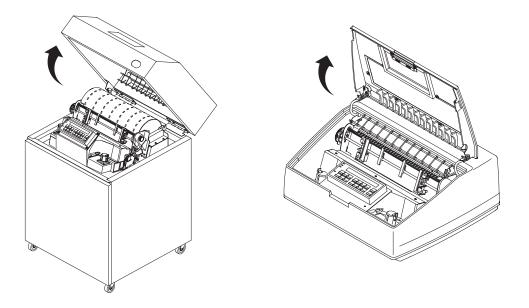
Figure 2–23. Opening the Printer Cover
