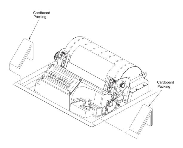
Figure 2–5. Removing the Cardboard Packing
