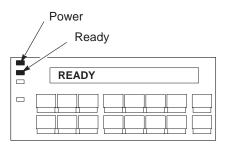
If there is a fault during the self-test, the Attention indicator lights and a fault message (such as "001 END OF FORMS") appears on the message display. See page 76 for information on fault messages.
