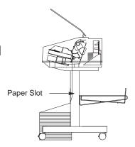
4 Pull the new paper above and behind the ribbon mask, but in front of the existing paper. (The ribbon mask location is shown on the ribbon path diagram.)
