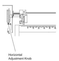
**13** Lower the forms thickness lever. Set it to match the paper thickness (refer to the note on the shuttle cover).
