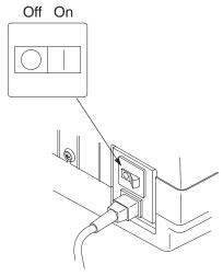
When you power on the printer, the Power indicator lights and the printer executes a power-on self-test. When the test successfully completes, the printer goes either to READY or NOT READY state, depending on the menu selection. In the READY state, the READY indicator lights and the message "READY" displays.
