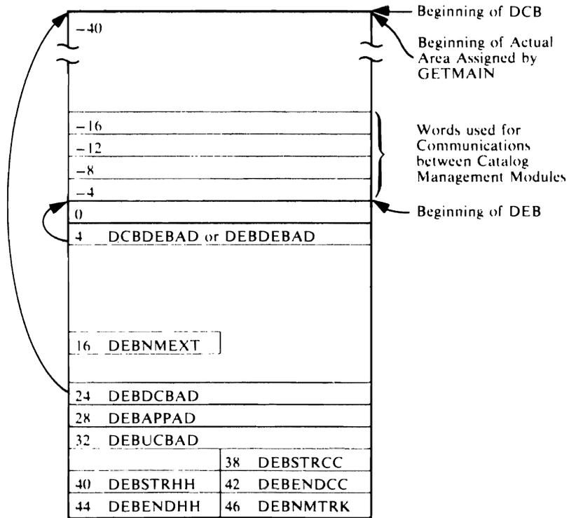
Figure 13. DCB/DEB Built by IGG0002H
