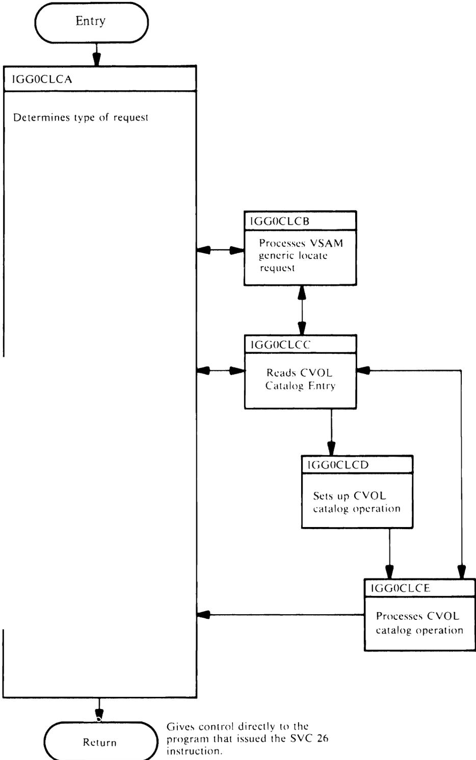
Figure 6. Overall Program Organization of the CVOL processor
