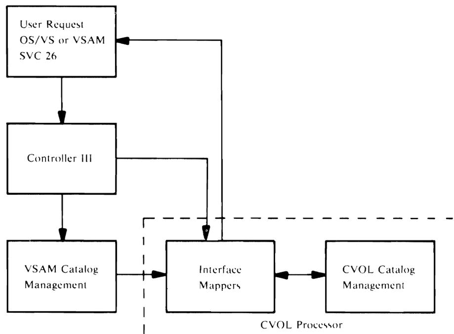
Figure 1. Flow of Control to the CVOL Processor
