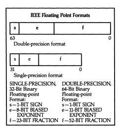
The Pascal and C Cross Compilers handle operations on single and double precision real numbers by generating calls to valuereturning functions from the run-time libraries. Calls are generated automatically whenever floating point operations, as listed, are encountered in the source code.
