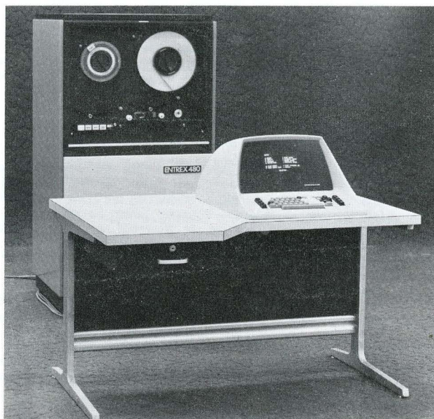
A System 480 CRT keystation is shown in front of the compact central control group.
