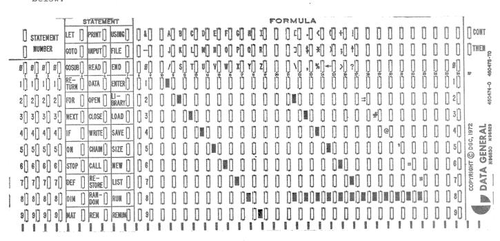
A stack of mark-sense cards may be read as a file and requires an EOF card at the end, which is a card with a single column in which all rows are marked. When in Batch mode, entire jobs may be entered from the card reader. Such card decks must conform to the Batch job control formats. Keyboard commands are suitable card input in Batch mode only. Consult with the System Manager for detailed Batch processing information.
