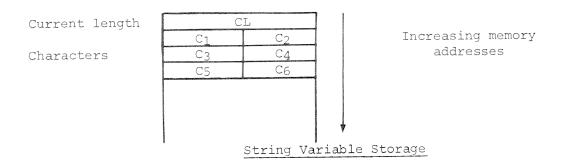
In the following examples, assume that A\$ is dimensioned to 10, and A\$ = "ABCDE". The current length of A\$ is 5.
