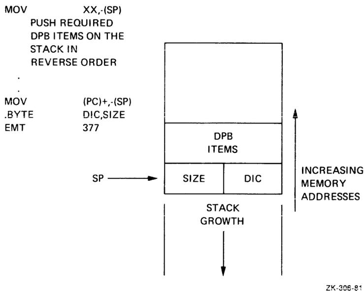
Figure 1-2 Directive Parameter Block (DPB) on the Stack
