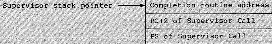
The stack, as shown, represents the stack content immediately after issuing the Supervisor Call directive. The user stack pointer is not guaranteed to remain valid.
