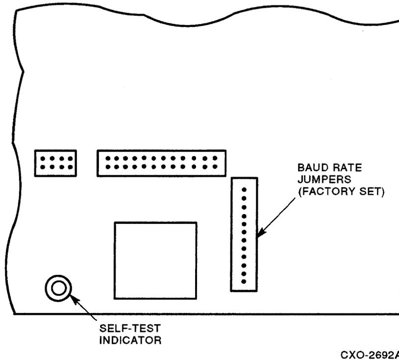
Figure 3-29 TU58 Baud Rate Jumpers
