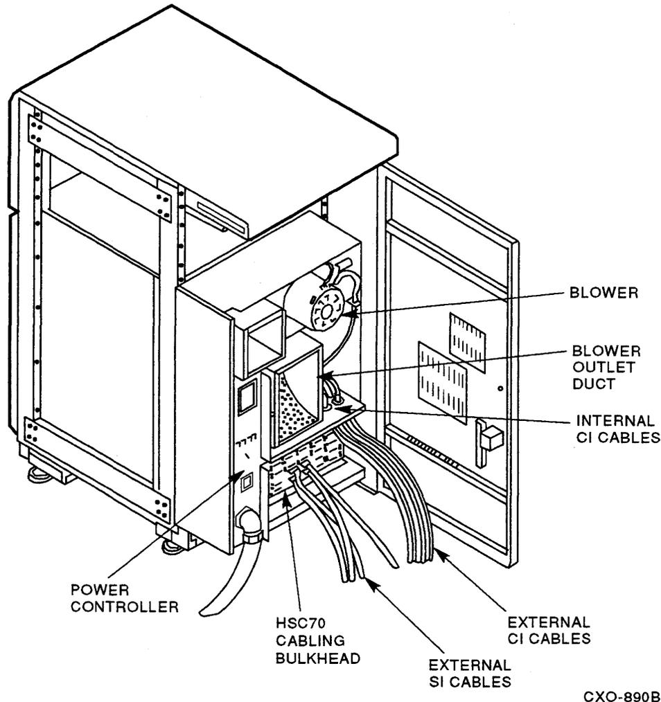
Figure 1-5 HSC Cabinet Inside Rear View
