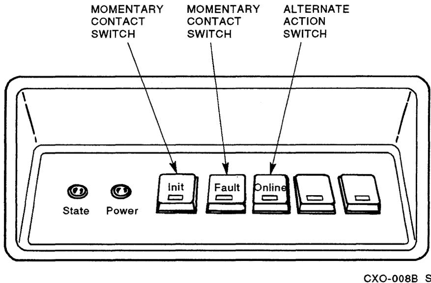
**Figure 2-1 Operator Control Panel**
