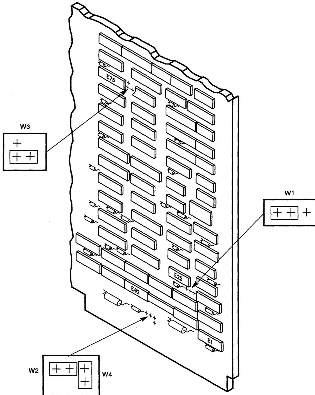
NOTE: BOXES INDICATE THE W1 AND W3 FAULT JUMPER POSITIONS. THE DEFAULT FOR JUMPERS W2 AND W4 IS "OUT".
