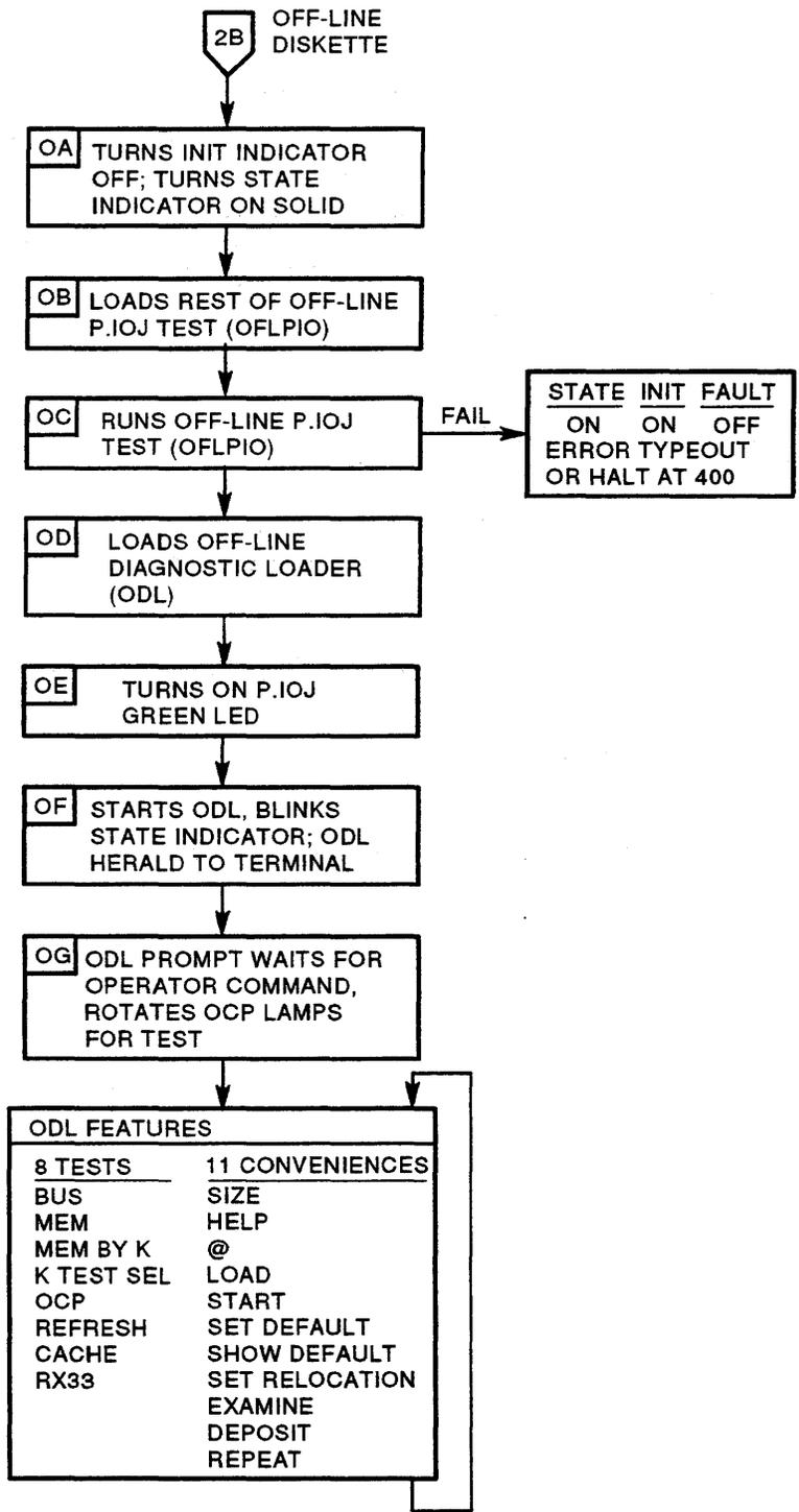
NOTE: FIRST PORTION OF THE OFLPIO TESTS WAS LOADED WITH THE PREVIOUS LOAD OF EIGHT BOOT BLOCKS.
