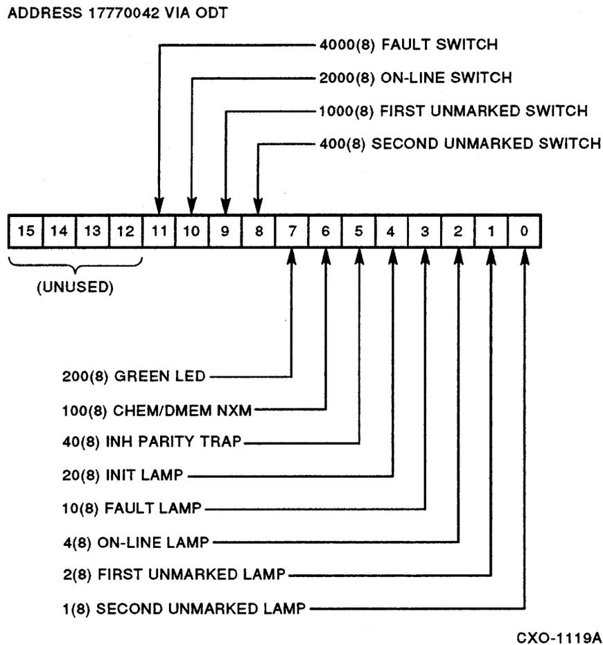
**Figure 6-1 P.ioj Switch Display Register Layout**
