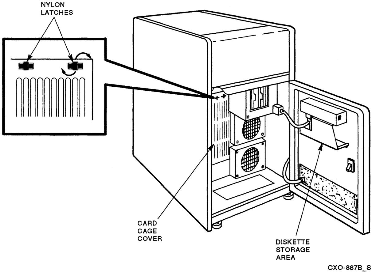
Figure 3-9 HSC Card Cage Cover Removal
