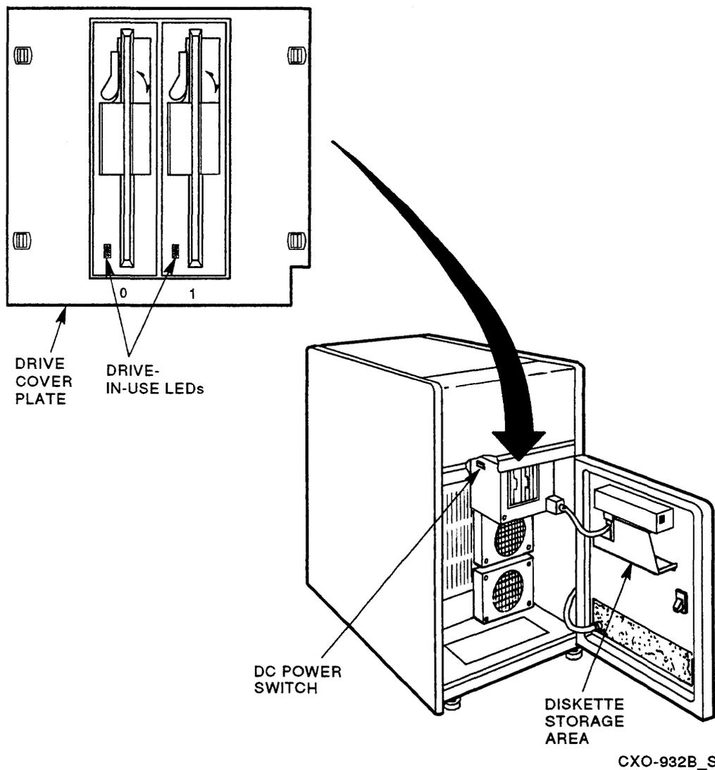
Figure 2-3 RX33 and dc Power Switch
