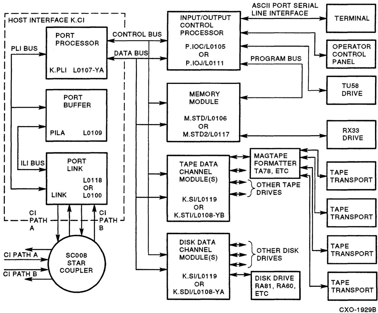
Figure 1-13 HSC Subsystem Block Diagram
