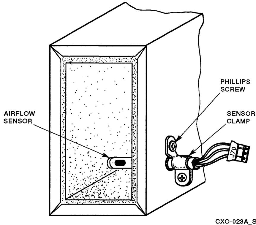
**Figure 3-35 Removing and Replacing the HSC50 Airflow Sensor Assembly**
