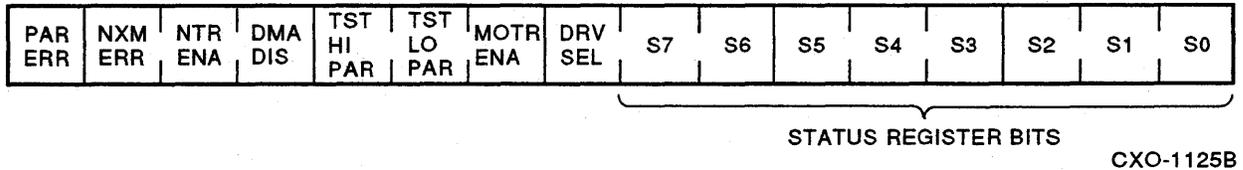
**Figure 8-24 RX33 Floppy Controller CSR Breakdown**
