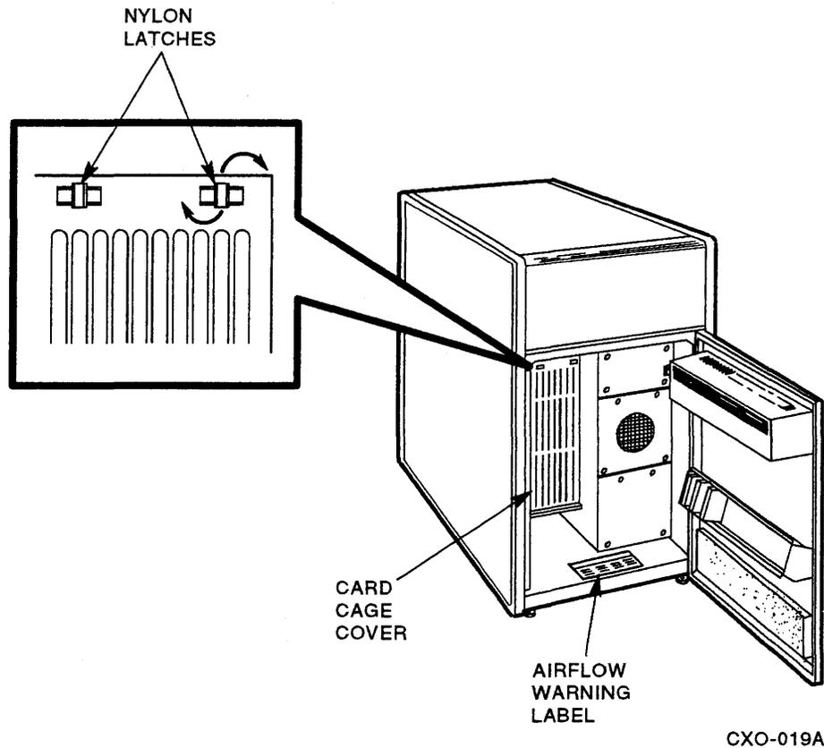
Figure 3-10 HSC50 Card Cage Cover Removal
