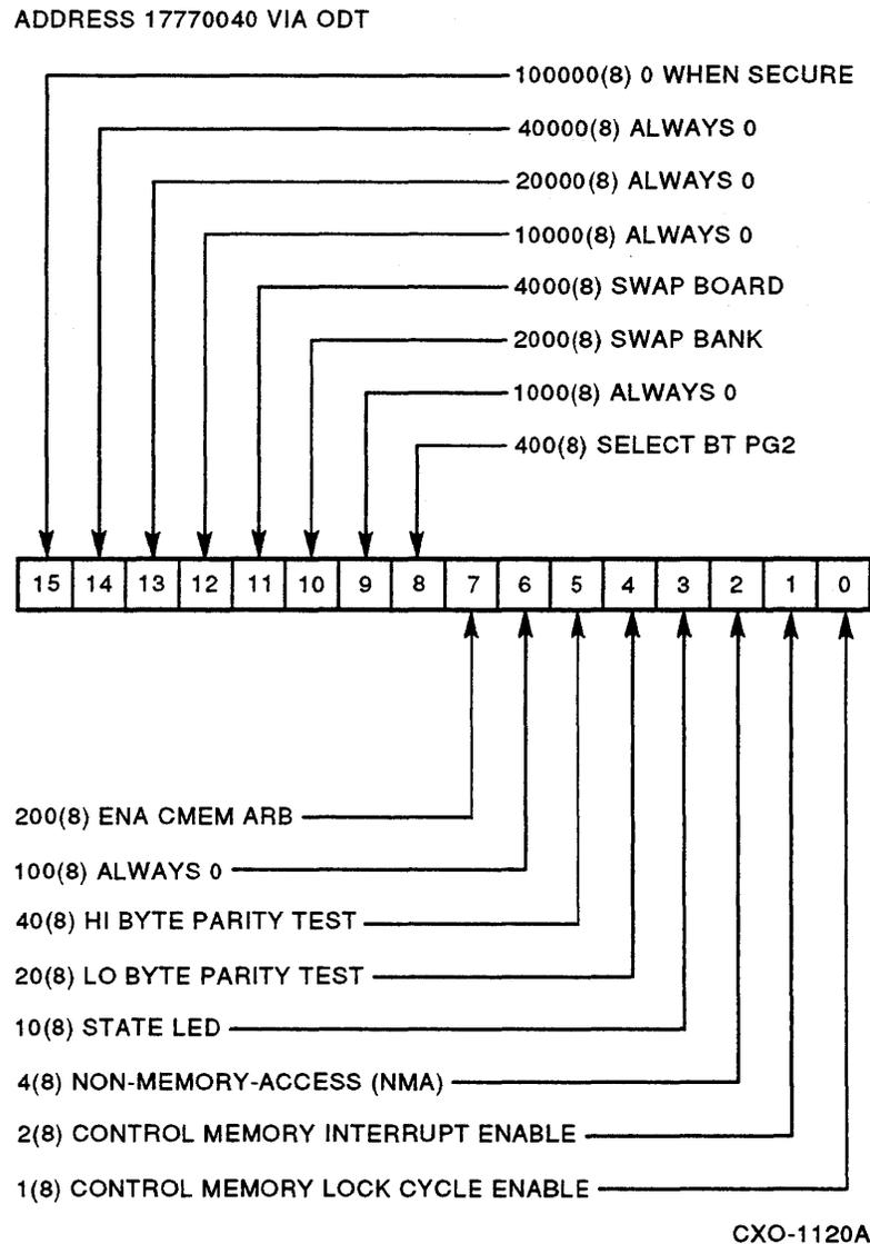
Figure 6-2 P.ioj Control and Status Register Layout
