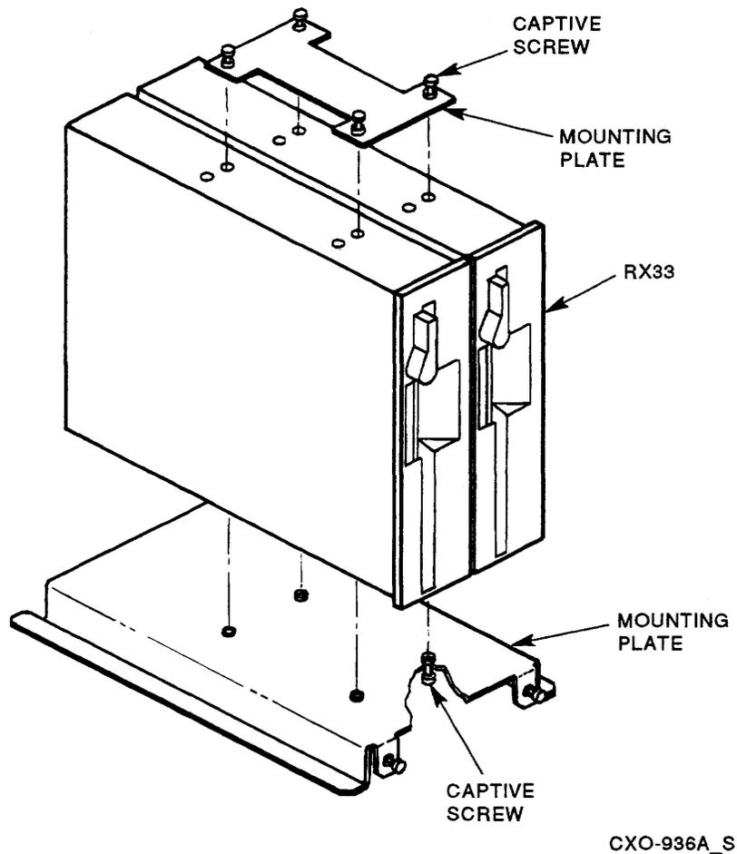
**Figure 3-22 RX33 Disk Drive Removal**
