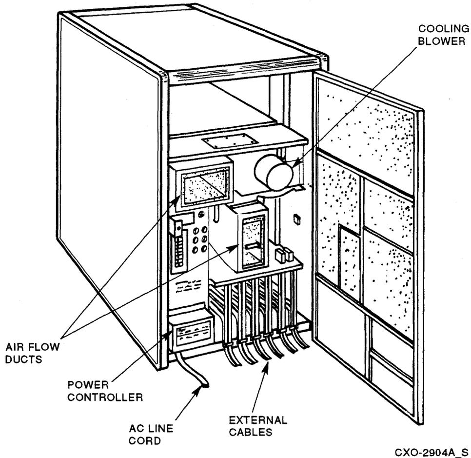
**Figure 1-10 HSC50 Cabinet Inside Rear View**
