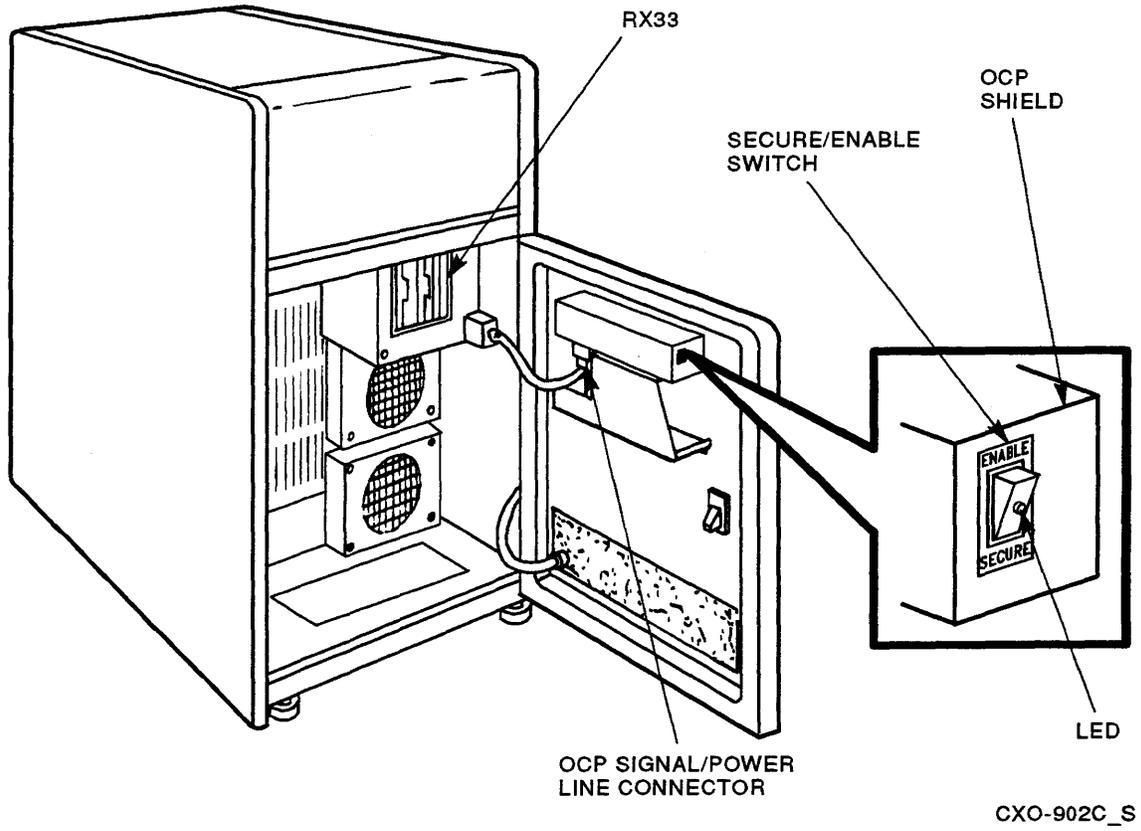
Figure 2-2 Controls/Indicators Inside Front Door
