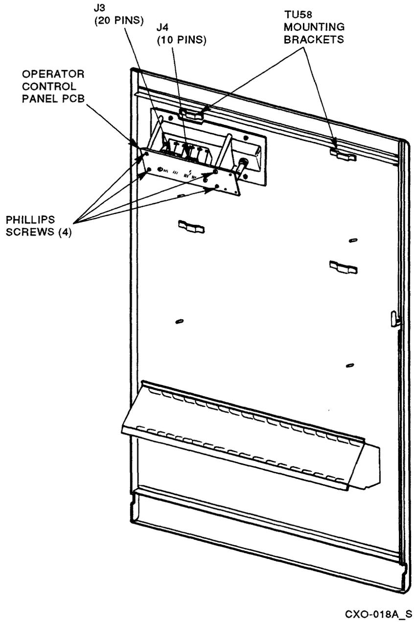
Figure 3-31 Removing the HSC50 OCP
