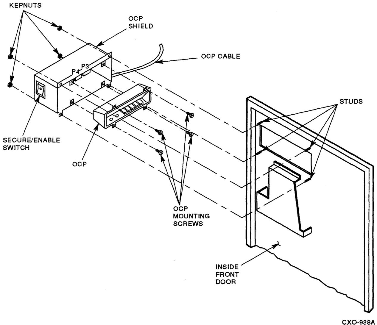
**Figure 3-30 Removing the HSC OCP**
