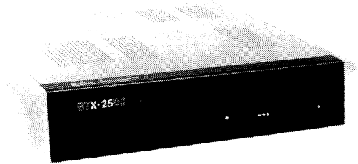
EDA Instrument's BTX.2500 is a microprocessor-based packet assembler/disassembler that enables users of Burroughs Poll Select Protocol to use CCITT X.25-based data networks.
