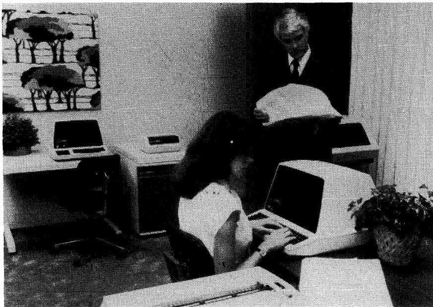
*The MAI/Basic Four System 210 features 64K bytes of main memory (expandable to 256K bytes in 32K-byte increments), a disk storage capacity of 57.4M bytes, and a cartridge tape drive providing 9.2M bytes of additional storage. Introduced in July 1981, the System 210 is available for \$25,740.*
