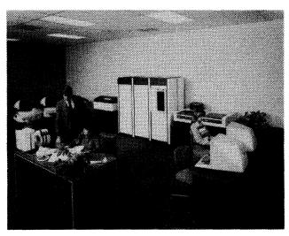
The BTI 8000 is one of the largest models shown in the specification charts, offering from 256K to 8 million bytes of main memory and from 33M to 8,000M bytes of disk storage. The 8000 will support up to 512 workstations, line printers, and reel-to-reel tape drives. The price of a basic system is \$86,850.
