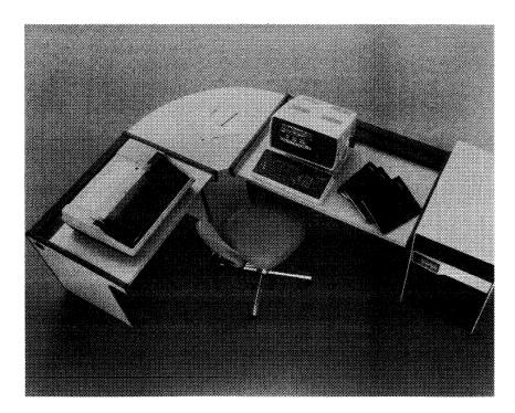
The Compal 9000 is built around a Data General MicroNova. With prices beginning at \$19,995, the 9000 offers from 64K to 128K bytes of main memory, floppy, cartridge, and fixed-head disk storage, serial and line printers, reel-to-reel and cassette/cartridge tape drives, and supports up to 16 CRT's.
