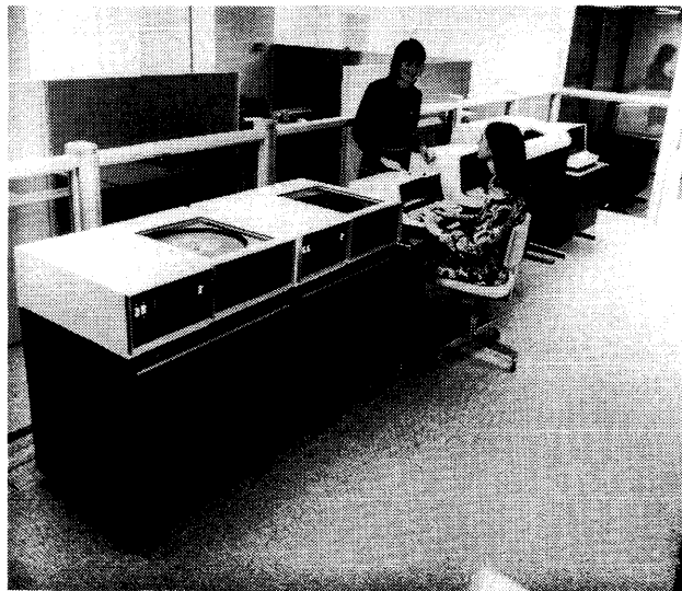
Another of the many faces of the world of minicomputers is illustrated by the Datapoint 5500 processor running a software package called Datashare. The combination supports up to 16 users simultaneously and provides each with the apparent full facilities of the computer. Not too many years ago, time-sharing was considered the province of large, highly specialized computer systems.
