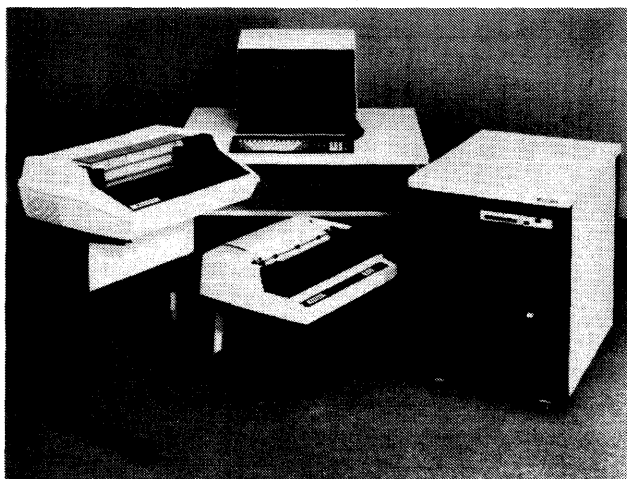
The Inforex Gen-V offers data collection and office automation in both centralized and distributed environments. As a multiuser, multitasking system, it supports up to 28 terminals which can be used for data entry, word processing, spreadsheet, and database management.
