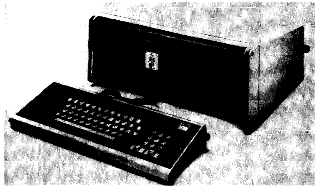
IBM provides an alternative to sophisticated software links with its 3270 Personal Computer. It acts as both a personal computer and a 3270 terminal, displaying both types of data simultaneously through windows.
