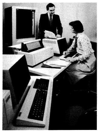
This Nixdorf 8870 configuration includes the processing unit with up to 512K bytes of main memory, two 40-megabyte cartridge disk drives, two display/printer workstations, and one 9-track magnetic tape drive.
