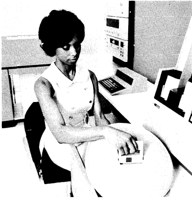
A drawer beneath the 5424 Multi-Function Card Unit houses the compact 5444 Disk Storage Drive and its removable single-disk cartridge.
