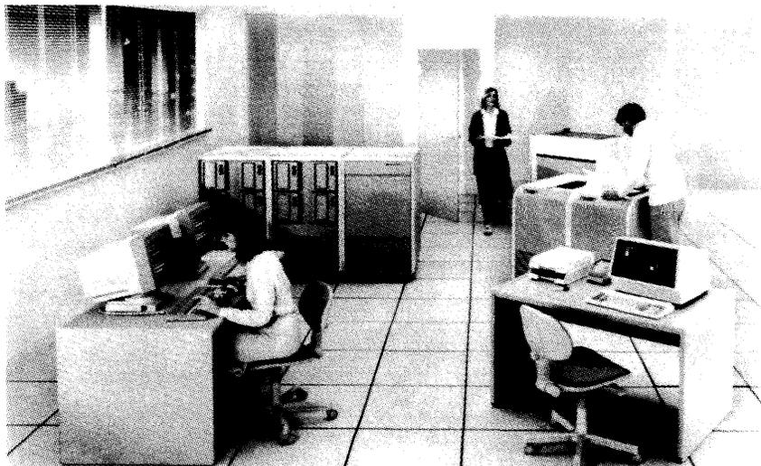
*The new Honeywell Bull DPS 7000 Series, the apparent replacement for the DPS 7 Series, is designed to handle high volume transaction processing and supports manufacturing and health industry applications. The Model 30, shown in the photo, is configured with eight 500-megabyte mass storage units, a 900 lines-per-minute printer, and a 1600/6250 bits-per-inch magnetic tape subsystem.*
