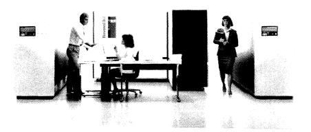
The Bull DPS 8000 Series, with one to four processors, spans the performance range between the DPS 8 Series and the DPS 90 Series. The maximum configuration contains four CPUs and 64 physical channels.
