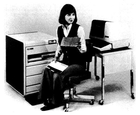
The DECstation 88/50 shown here is one of the business-oriented DEC-station systems that range from an LSI-based 16K word video data processor version with one megabyte of floppy disk storage to a 32K word PDP-8/A version with ten megabytes of disk-pack storage. Software for business and general-purpose program development is available. DECstations range in price from \$8,250 to \$25,100 with quantity discounts available at all levels.
