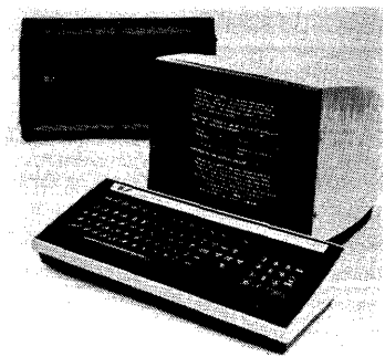
Three faces of CRT terminals. The IBM 3270 Information Display System, illustrated on the left, is a replacement for the prior IBM 2260 and 2265; it features high modularity and expanded capability. The Datapoint 3300, shown in the middle, can replace a Teletype Model 33 or 35 in a time-sharing network or other application; it has also been picked up by a number of manufacturers for inclusion in larger systems. The Four-Phase System IV/70 on the right includes a powerful programmable controller (background) for sophisticated applications.
