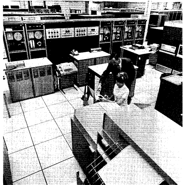
Multiple Honeywell computers in a "supercenter" in Cleveland provide the computing power for users of the General Electric Company's international Information Services Network.
