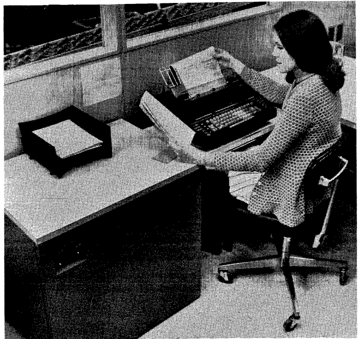
Two ways to implement intelligent terminal capability by IBM. The IBM System/3 Model 6 on the left is a keyboard oriented version of the general purpose Model 10; an interface can be attached for communications with larger IBM computers. The 3735 Buffered Terminal on the right is a disk-based, record-oriented, programmable terminal primarily aimed at automating forms preparation.
