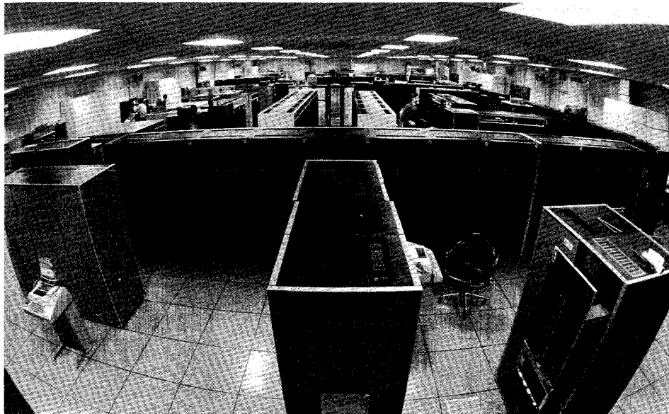
This panoramic view shows the eight DEC PDP-10 computers, configured in pairs, that provide the processing power for Applied Logic Corporation's AL/COM Time-Sharing System.
