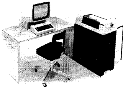
Three faces of CRT terminals. The IBM 3270 Information Display System, illustrated on the left, is a replacement for the prior IBM 2260 and 2265; it features high modularity and expanded capability. The Datapoint 3300, shown in the middle, can replace a Teletype Model 33 or 35 in a time-sharing network or other application; it has also been picked up by a number of manufacturers for inclusion in larger systems. The Four-Phase System IV/70 on the right includes a powerful programmable controller (background) for sophisticated applications.
