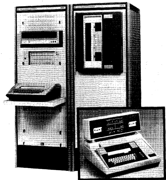
Texas Instruments continues to develop its thrust into systems to complement its large components business. The Electronic Message Switching System II (EMS II) is intended for free-standing store-and-forward applications. The inset in the lower right corner shows TI's latest version of its Silent 700 terminal; this one includes a pair of cassette tape units to provide ASR capability.
