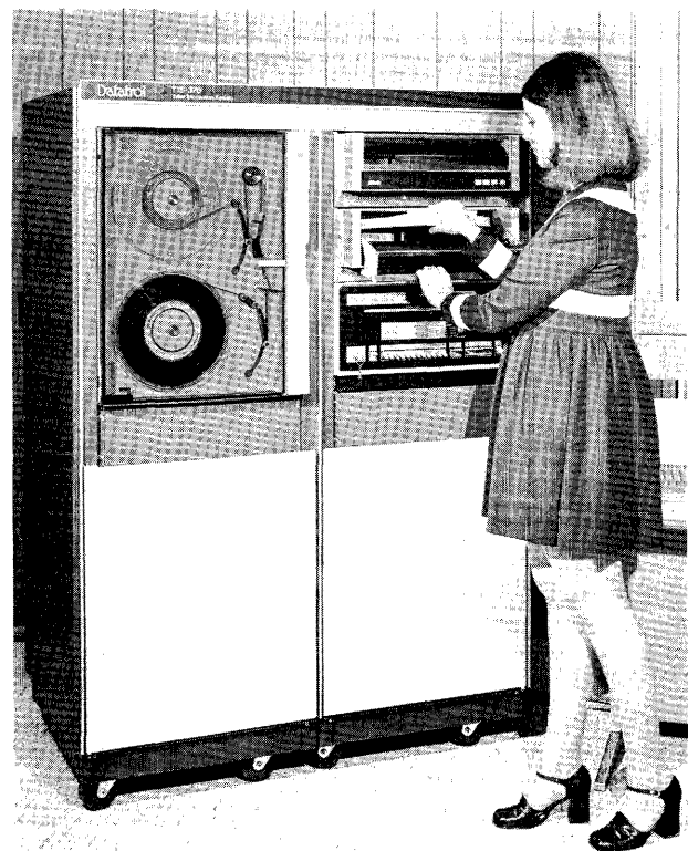
This system from Datatrol Inc. is representative of one of the most popular uses for voice response. It provides bank tellers with access to information about customers with just a telephone at their window - which they normally have anyway.
