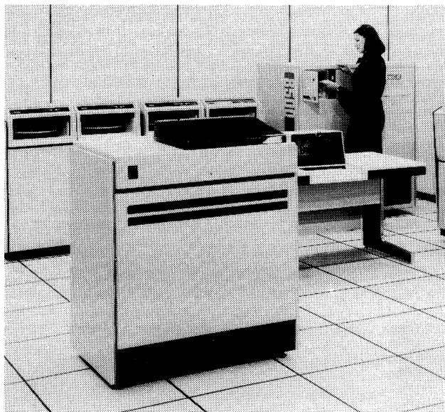
The NCR 721 (foreground), depicted here with an NCR Criterion 8500 mainframe, features a readily accessible control panel and dual cassette unit (on top of unit) for program loading, data input, and memory dumping.
