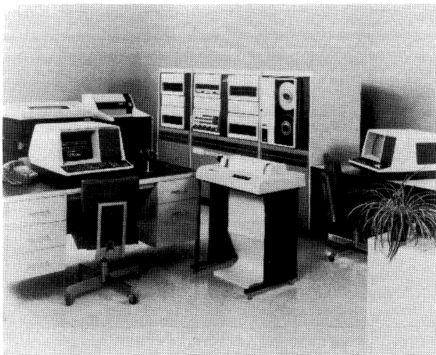
The top-of-the-line PDP-11/70 processor is shown above surrounded by peripheral devices. When DECnet is fully installed, the peripherals can operate as if they were attached to other remotely-located processors included in the DECnet network.
