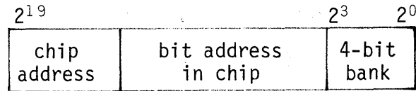
Figure 5-1. Memory address; 16 banks
