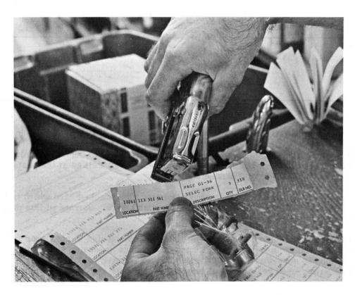
PICKING LABEL IS ATTACHED TO PARTS. THE LABEL LISTS THE BIN NUMBER (at left), THE PART NUMBER, THE DESCRIPTION, THE QUANTITY AND THE DEALER NUMBER. THE LABEL IS CHECKED AGAINST THE PACKING SLIP PRIOR TO SHIPMENT.
