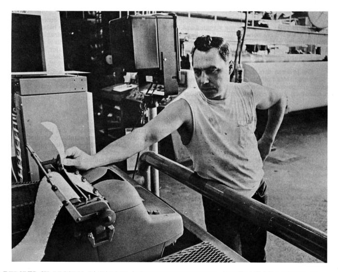
REPORTS ON PROCESS VARIABLES AND INSTRUCTIONS FOR ADJUSTING THE PAPER MA-CHINE ARE ISSUED BY COMPUTER AND PRINTED OUT.
