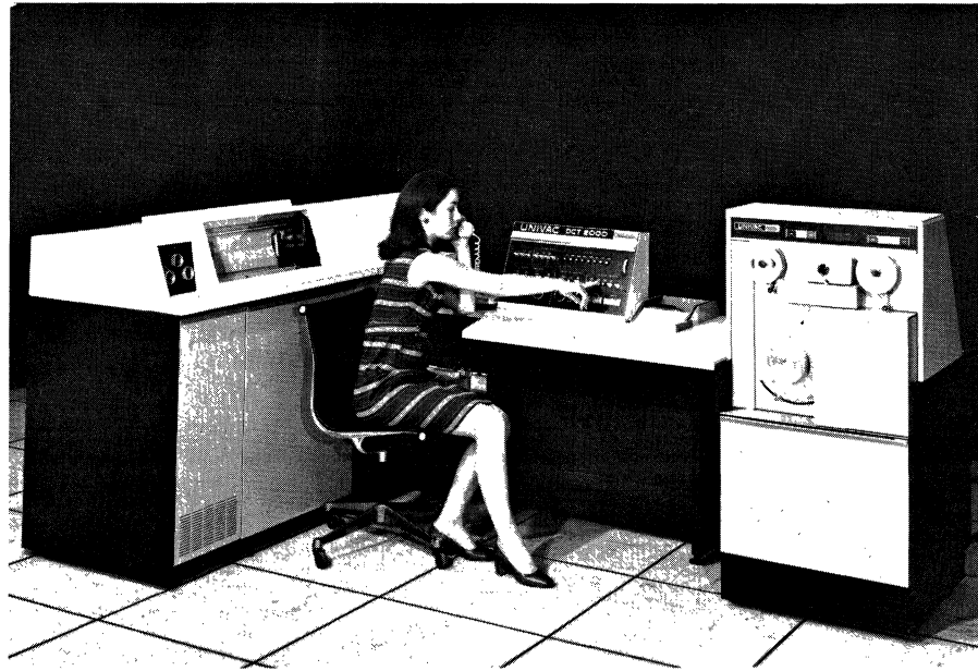
Figure 1. The UNIVAC DCT 2000 Data Communication Terminal Shown With the Paper Tape Subsystem (right).
