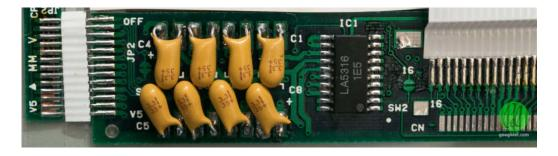
Unfortunately, when reassembling, I found a slight interference between C5 and the plastic frame, so a little bit of a snip was needed.
