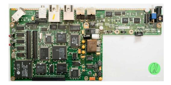
In the end, it's probably not my best work, but it's **my first attempt at SMD work** with a single iron. It's not ideal, but functionally, it should be **just fine**. The larger capacitors weren't available in tantalum, so I settled to go with one solid-electrolytic and a regular 105 degree rated electrolytic. It's a compromise I had to make.
