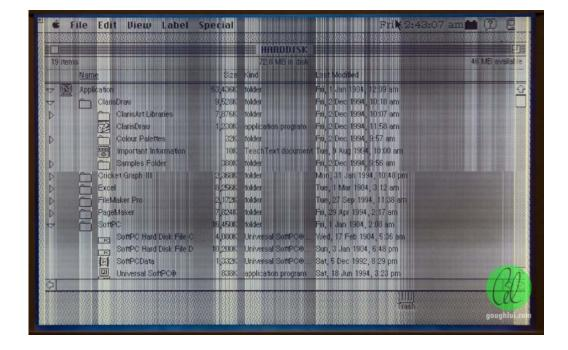
At this point, I was a bit annoyed and disappointed that my time investment didn't cure the machine entirely. The screen still exhibited column interference and occasional blanking of the bottom-third. I suspect this may be a problem with one of the chips on the flex cables to the array, as when the unit is cold, it is reliably clean and only plays up as it warms up.
