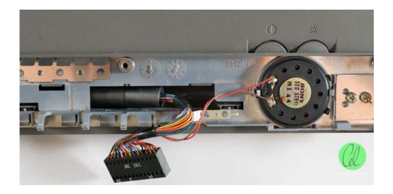
With that major piece out of the road, the next stop was the display – a known troublesome part in my case. To get to it involved removing the Sony speaker from the body, clutch plate, clutch covers, brightness and contrast knobs, more screws and screw covers etc.
