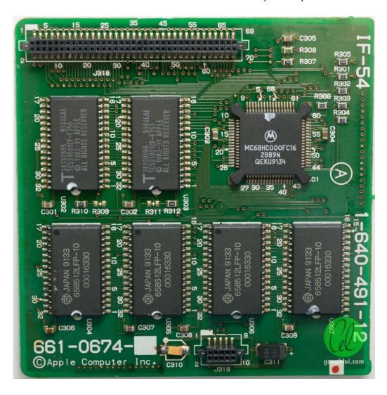
The capacitor (C310) was replaced with an equivalent value SMD tantalum capacitor — noting that the band on tantalum capacitors faces the **positive**. The orientation is a bit crooked, but considering I'm doing it by hand with a single iron, I think it's okay.
