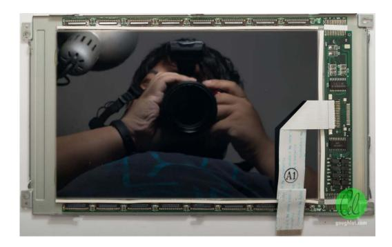
We can see the flat-panel chip-on-flex drivers top and bottom. The flexible flat cable was very carefully threaded out from the frame — it's not on a connector on the PCB side which makes it both fragile and annoying.
