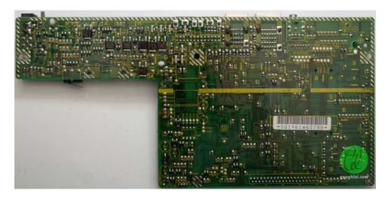
The underside of the board after it was repaired, and it looks mostly the same. The original factory seems to have left some sort of flux or coating on the rear which isn't really a nice conformal coating or anything, but it gives it an uneven glossy appearance.
