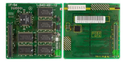
This would turn out to be our first patient, as this has an SMD electrolytic capacitor near the small connector. The tantalum next to it doesn't necessarily need replacement.
