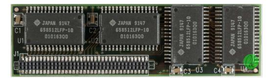
The pSRAM in question is a Hitachi 658512LFP-10. I managed to find some for sale online, but in a larger batch than I needed and at a price I'm not sure I could justify — after all, to do the modification could risk damaging the board as it stands, and I'm not entirely sure if it would work. The capacitors on the board look like they're not the right size for the footprint, hence their "crooked" orientation. No caps need replacing here, which is good.
