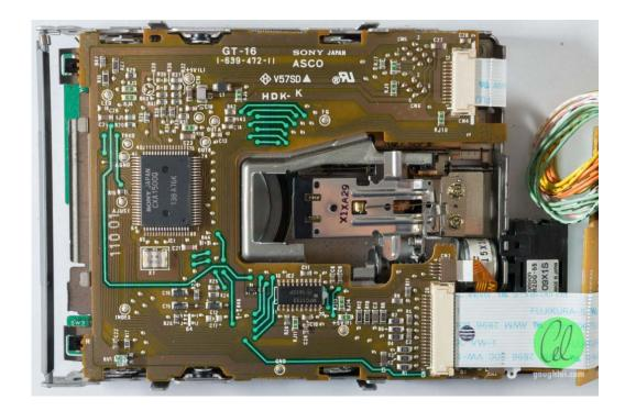
Taking a peek under the shell shows a clean drive, with a PCB on the top and no obvious signs of electrolytic capacitors. There's one adjustment potentiometer in the bottom left which *might* be for drive speed? Who knows. I'm not touching it ... until I have to.
