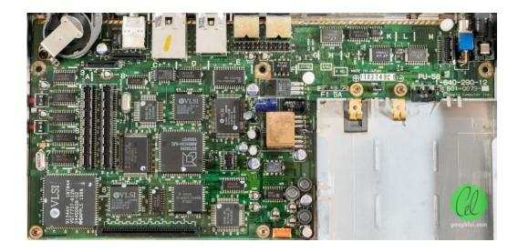
The next step is the main-board, which has a whole lot of capacitors that look like they need attention. The surface mount electrolytics show signs of distress, namely the solder joints around them look a little corroded, indicating that there is probably some leaking of electrolyte over time.
