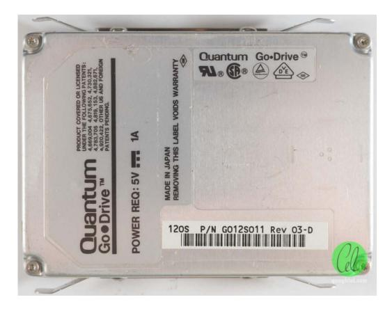
Sadly, these are known to be failure prone nowadays, because of their internal rubber parts which have also probably disintegrated into goo.
