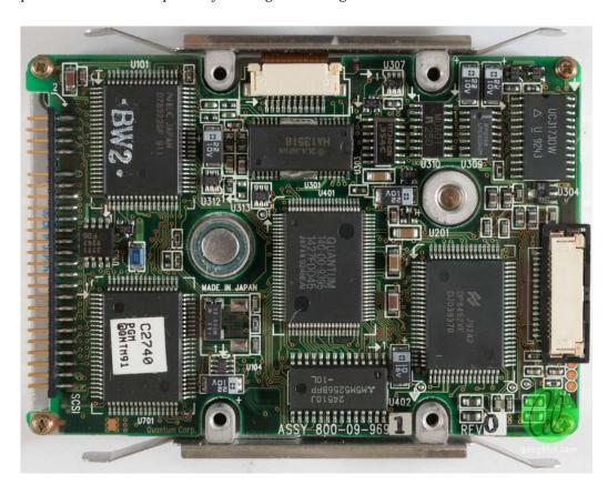
The underside has a few chips which take up the majority of the area of the board. No electrolytic caps that I can see, which is good.
