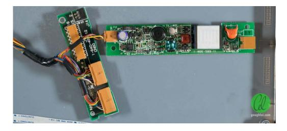
The backlight inverter had two electrolytic capacitors, which might need replacement. I decided to be safe and replace it anyway — although the replacement tantalums were a bit tall even when bent over, resulting in some stress on the board when reassembled.
