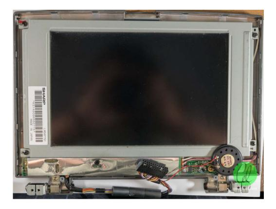
Inside, I found a Sharp LM64P791 LCD screen. There is a connector board and LCD backlight inverter underneath behind the shielding.
