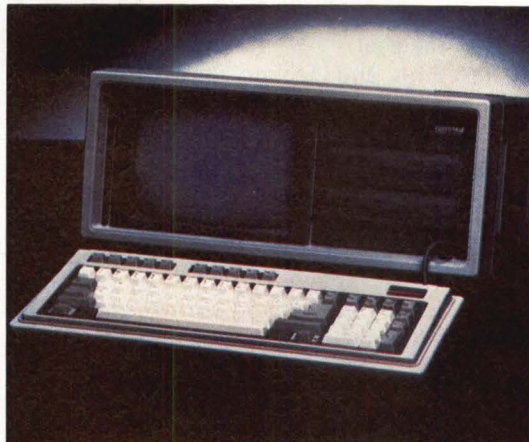
Supporting up to 4M bytes of internal RAM memory, the Compaq Portable II uses a 6-MHz 80286 and operates as a single-user workstation.
