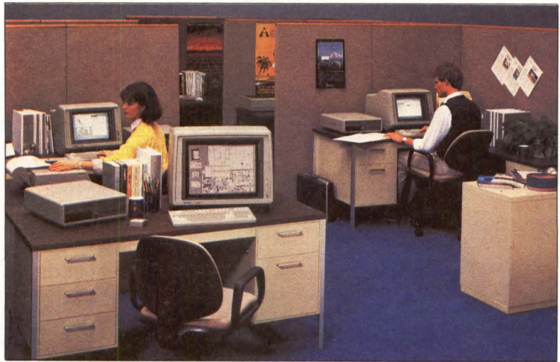
Three artificial intelligence workstations from Tektronix run Smalltalk, LISP and Prolog. They are the 4406 (foreground), 4405 (back left) and 4404 (back right).
