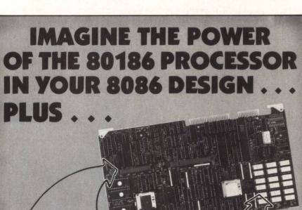
two iSBX connectors for adding serial, parallel, SCSI, or IEEE 488 I/O interfaces; A/D or D/A converters' or other Multimodule boards.
