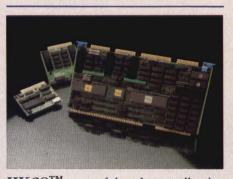
HK68TM powerful and versatile single board UNIX<sup>TM</sup> (System III or V) or CP/M68K<sup>TM</sup> system with 68000/68010 CPU (8Mhz or 10Mhz), MMU, quad channel DMA, four serial ports, 128K, 256K, 512K or 1M bytes of on-board RAM with parity, up to 32K bytes of on-board EPROM, user acces-
