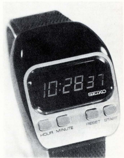
Numerals. Seiko's all-electronic watch drives liquid crystals with C/MOS circuits.
