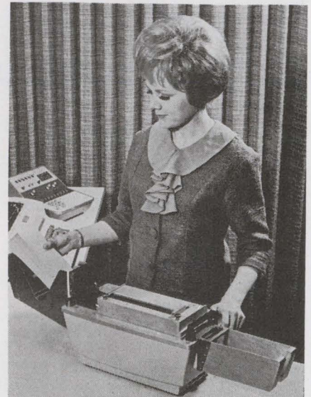
Unpunched cards. Machine writes and reads data entered on cards in the form of a magnetic code.
