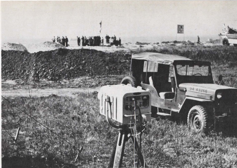
Amphibious tests. The Army put a prototype of the transceiver through its paces in ship-to-shore tests near San Diego, Calif. The service removed the scanning antenna to increase portability.
