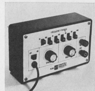
Compact digital pulse generator PG610 provides output pulses at repetition rates from 10 hz to 2 Mhz in six overlapping ranges. Output is compatible with TTL, DTL and RTL logic levels. It can be operated at high output pulse duty cycle. Dimensions are 2 x 3.75 x 6.25 in. Price (4-9) is $98.60. Computer Products, 2801 E. Oakland Park Blvd., Fort Lauderdale, Fla. 33306. [368]
