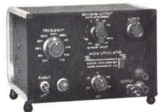
Type 1311-A . . . $225 in U.S.A. • 11 fixed frequencies, 50 Hz to 10 kHz • 1-watt output • Distortion typically <0.1%
