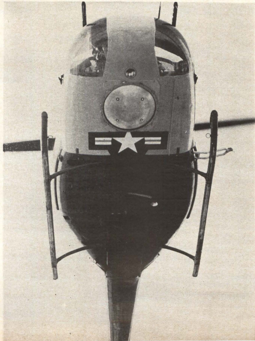
Circular pod of acoustic sensors fixed to the bottom of a helicopter picks up sonic boom of projectiles to warn pilot of small-arms attack
