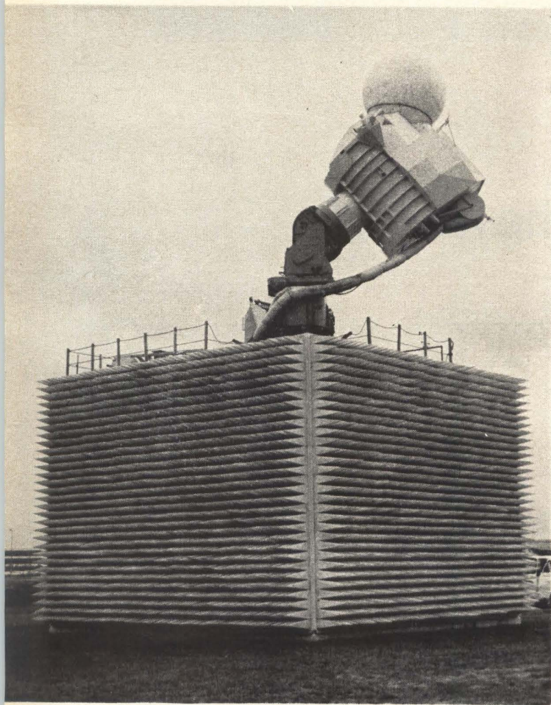
Rendezvous radar inside radome is evaluated at the Manned Space Flight Center's antenna range. Setup includes a model of Lunar Module to determine what effect the LM itself will have on the radar.
