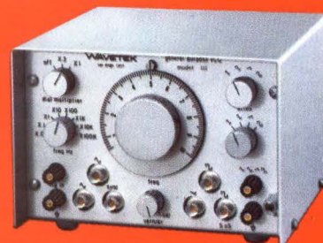
Wavetek Model 111 VCG generates sine, square, triangle, and ramp waves from 0.0015 Hz to 1 MHz, and offers precision control of the frequency of the waveforms by external voltage.
