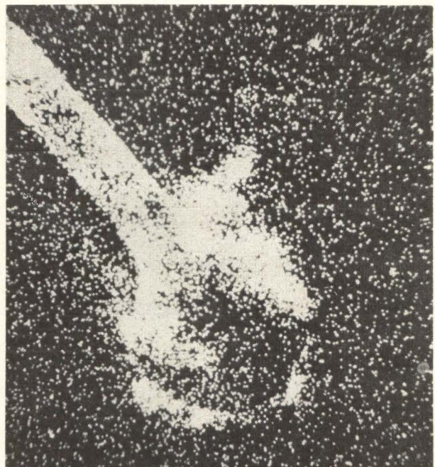
Electron microprobe scan of lead and pad area on IC surface discloses presence of contaminants. The frequency and intensity of X-rays returned from the IC surface identify the contaminant material, chlorine in the lower photo, carbon in the other.
