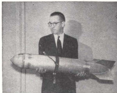
BOMB-SHAPED transmitter is fitted in flight with vertical 10-ft dipoles above and below, and a 16-foot trailing dipole
