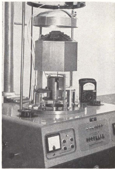
ONE-SHOT process equipment (left), shown with vacuum chamber removed, deposits films on several substrates with one firing of source material. Diagram (center) shows details of substrate holder and general location with respect to source material. Geometric diagrams (right) are used to accurately position holder with respect to source material in accordance to material used; note also modifications in shape of holder's support frame to accommodate silicon monoxide deposition—Fig. 1
