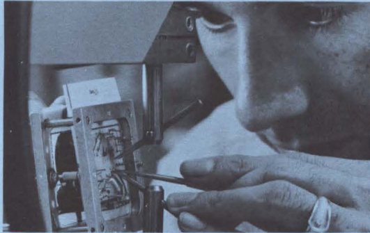
Welded module construction
