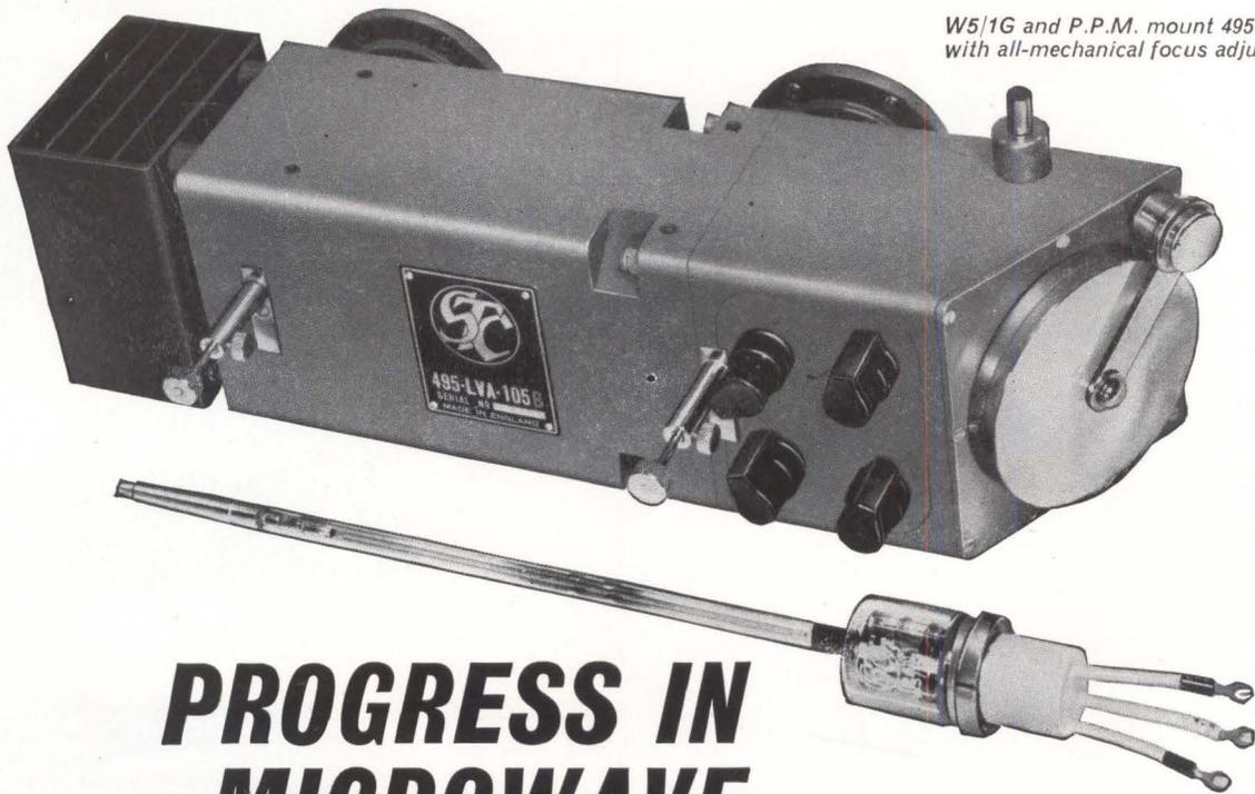
W5/1G and P.P.M. mount 495-LVA-105B with all-mechanical focus adjustment.
