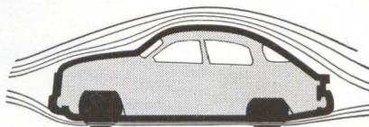
**SAAB BODY SHELL** is designed and wind tunnel tested for best possible aerodynamic efficiency. Full belly pan further reduces wind resistance and subdues road noise. Result: increased economy, better performance, excellent stability—even in cross-winds of gale force. Moreover, the SAAB body shell is virtually uncrushable, combining 18- to 20-gauge steel (thicker than most American cars) and rigid unitized construction for optimum safety.
