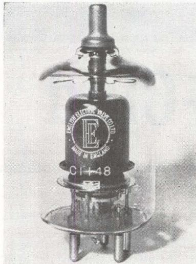
**Pulse Modulator for High Output Radar**
